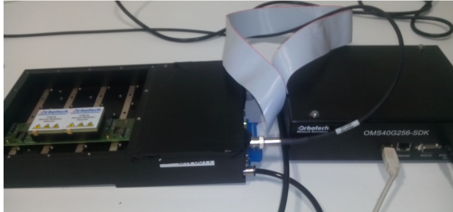
Figure 5.4: OMS Detectors Array Unit and the data collection unit OMS36G256-SDK
