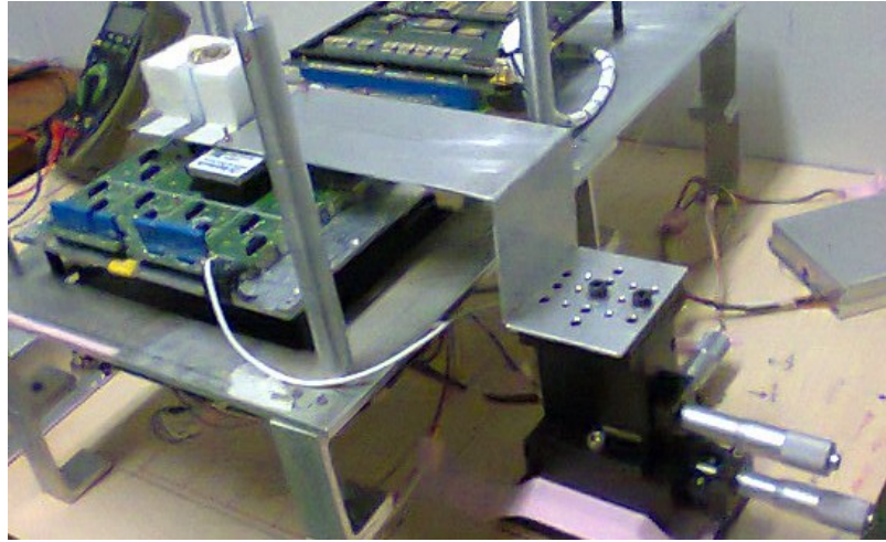
Figure 5.8: Experiment setup for Crosstalk experiment. The pixels were illuminated by source through a narrow slit to localize the pixel position.
