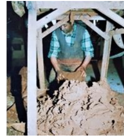
Figure 19, 20. Kneading with electric valse
