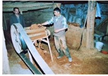
Figure 19, 20. Kneading with electric valse
