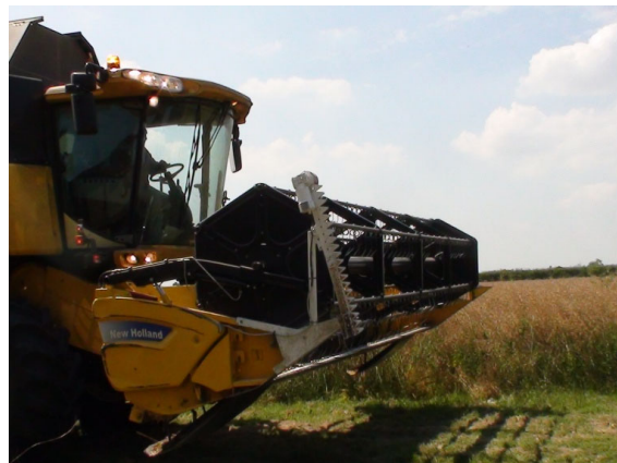
Figure 2. Modified wheat header for canola harvesting (photo by Authors).
