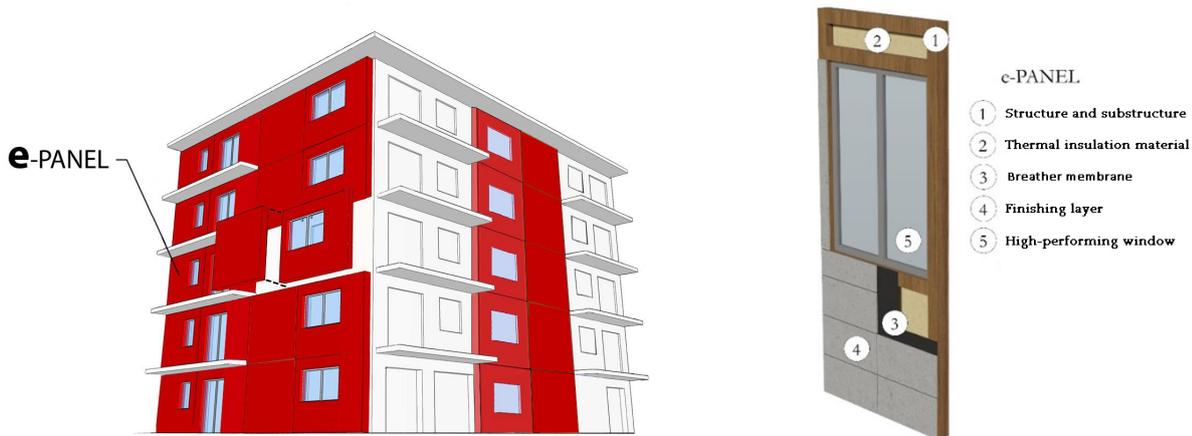
*Figure 1. e-PANEL application on the facades and its stratification*
