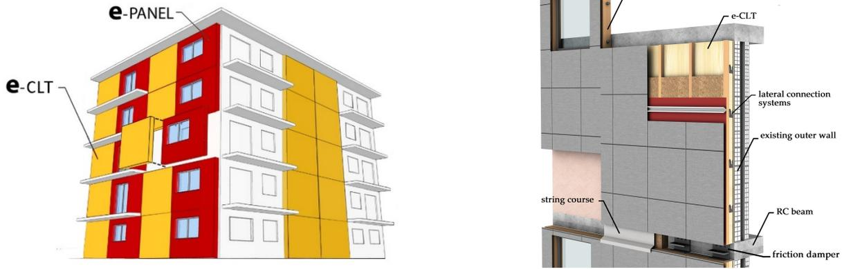
Figure 2. e-CLT application on the facades and its stratification
