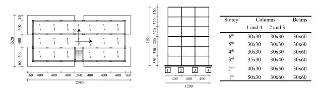
Figure 18. Features of the analysed RC frame: (a) Plan layout of the building, (b) geometrical scheme of the frame, (c) cross-sections of the frame members
