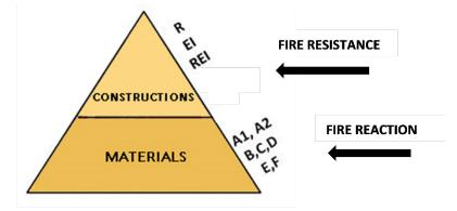
*Figure 14. Fire reaction and fire resistance classification according to EN 13501-1 and EN 13501-2*
