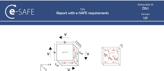
Figure 12. Representation of shear stresses on an infinitesimal CLT element [62]
