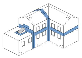
Figure 15. Example of separating fire-resistant façade bands between building compartments
