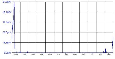
*Figure 16. Interstitial condensation for wall ID4 in Climate Zone F – Vapour concentration class 3*
