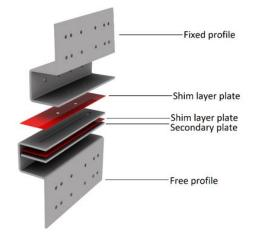
Figure 10. Schematic representation of friction damper design
