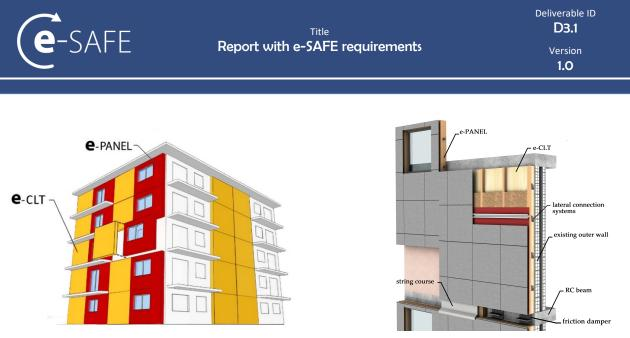
Figure 2. e-CLT application on the facades and its stratification
