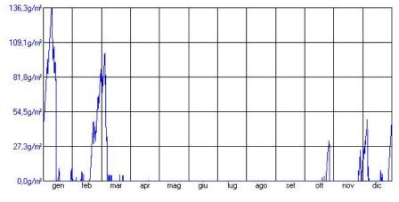
*Figure 17. Interstitial condensation for wall ID4 in Climate Zone F – Vapour concentration class 4*
