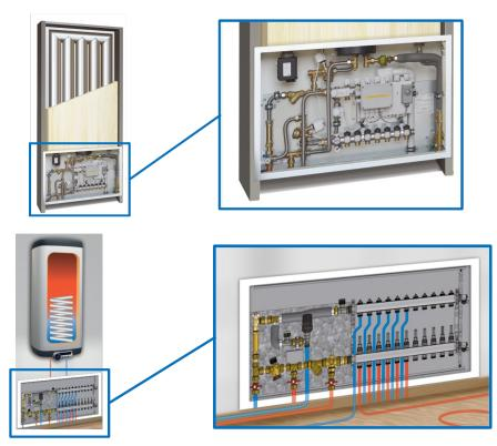
Figure 6. Prefabricated hydraulic units for different e-TANK configurations (flat on top and cylindrical at bottom)
