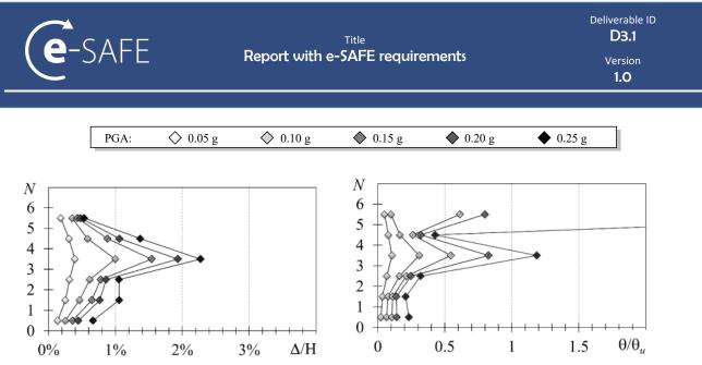
Figure 19. Height wise distribution of story drift angle of the frame (on the left) and chord rotation demand to capacity ratio of columns for NC limit state (on the right)
