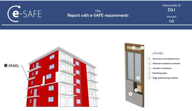
Figure 1. e-PANEL application on the facades and its stratification
