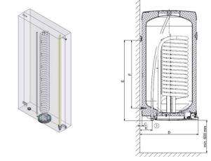
Figure 5. Flat (on the left) and cylindrical (on the right) e-TANK solutions
