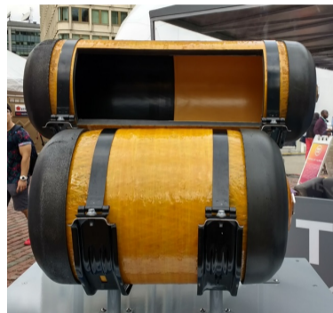
700 bar \text{cH}_2 tanks onboard Toyota Mirai
