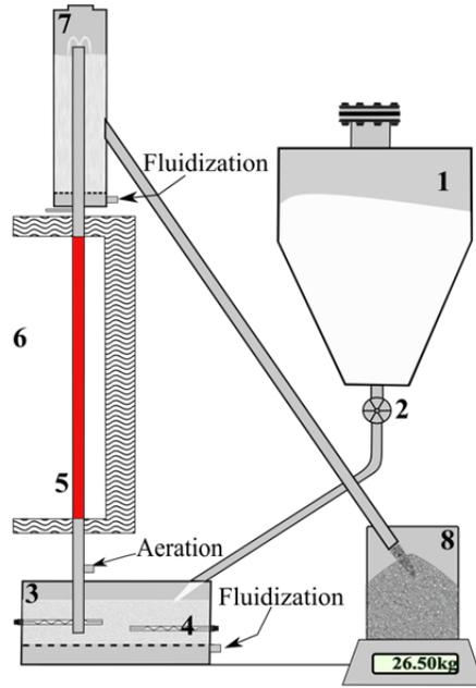
**FIGURE 1.** Experimental set-up cut view. 1. Hopper, 2. Rotary valve, 3. Dispenser Fluidized Bed (DIFB), 4. Electrical resistances, 5. Absorber tube, 6. Receiver cavity, 7. Collector Fluidized Bed (ColFB), 8. Container placed on weighing scale.
