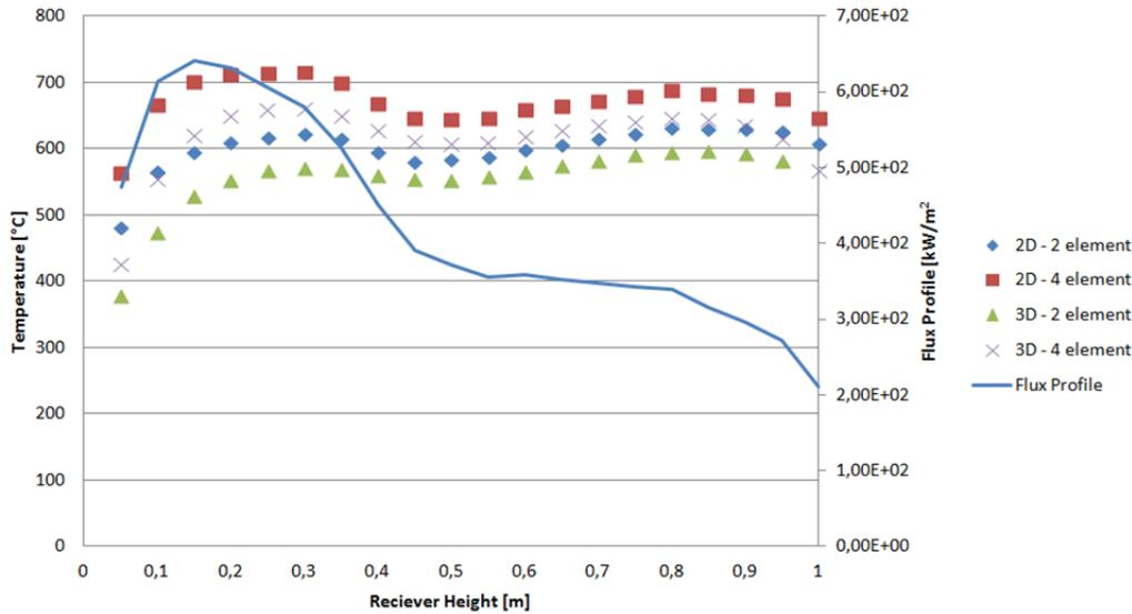
**FIGURE 3.** Applied solar flux and maximum tube temperatures (finned tube, cristobalite, 260 kg/h, and 243°C of preheating)
