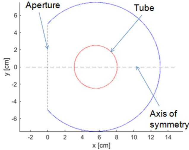
FIGURE 2. Top view of receiver geometry
