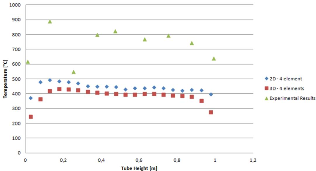
**FIGURE 4.** Maximum tube temperatures using a smooth tube with cristobalite flowing at 381.6 kg/h, and no preheating
