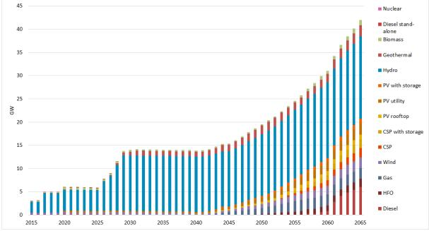
Figure 37. Power generation capacity by technology (GW) in the Slow Down scenario.
