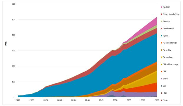
Figure 41. Electricity supply mix by technology (TWh) in the New Policies scenario.
