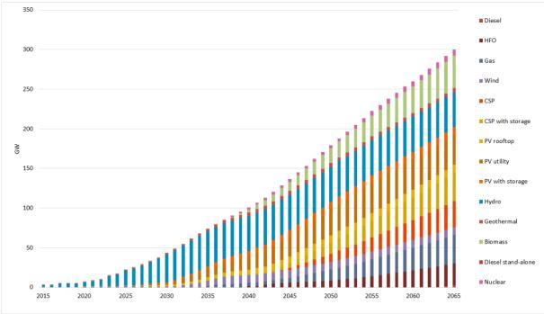
Figure 40 Power generation capacity by technology (GW) in the Ambition scenario
