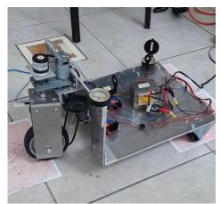
FIGURE 3: Vehicle used showing the tricycle topology.
