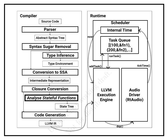
Figure 1. Architecture of *mimium* compiler and runtime.
