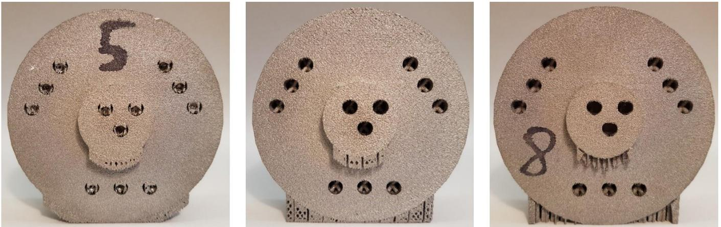
Figure 91: examples of three different types of support structure geometry used within EB-PBF, image credit: NSTP3-PF2-008 team.
