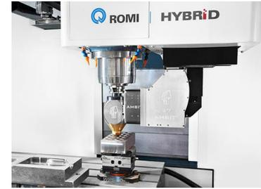
Romi CNC milling machine equipped with an Ambit DED head developed by Hybrid Manufacturing technologies.
