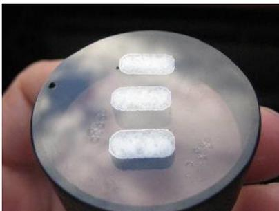
Nickel plating on a Polymer Powder Bed Fusion part
