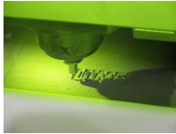
Matsuura combines the PBF process with CNC milling in their LUMEX Advance-25 machine to produce tooling with internal cooling channels
