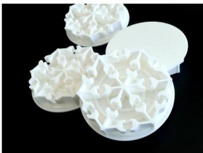
Alumina Oxide mirrors printed by Vat Photo Polymerisation
