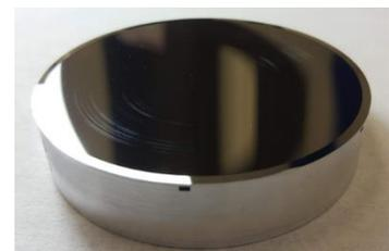
The aluminium substrate after diamond turning.
