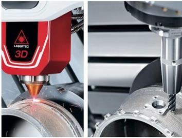
Direct Energy Deposition (DED) Laser cladding process combined with CNC 5 axis milling.
