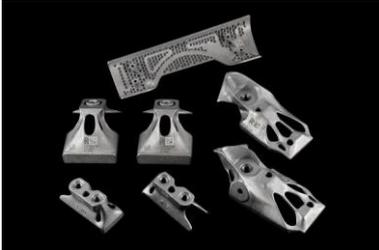
Metal components produced by metal PBF in AlSi10Mg4
