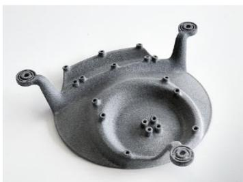
Rear side of the 3D printed FAME Active mirror concept.
