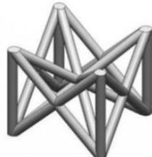
Face and Body Centred Cubic (BCC) with Z struts unit cell
