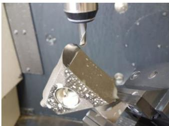
Subtractive processing of the printed part. In a second milling step, the fixture will be removed.
