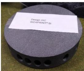
Manufactured by SGL CARBON, supplied by TNO in Sicaprint® Si (Si-SiC)
