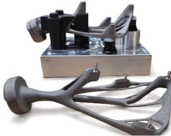
(Photocurable) adhesives, wax or hot melts can be used to keep the AM part in place during post processing
