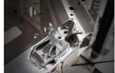
Welding the aluminium parts to the chassis of a Roll-Royce Ghost car body
