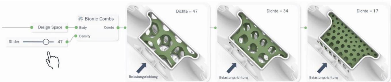
**Figure 63: Bionic Algorithms – By using a parameter slider the input values are altered. The design is re-calculated and automatic redrawn. Image credits: ELISE GmbH.**
