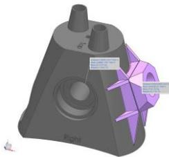
Parts can be equipped with an additional handle in the CAD file on a non-critical place.
