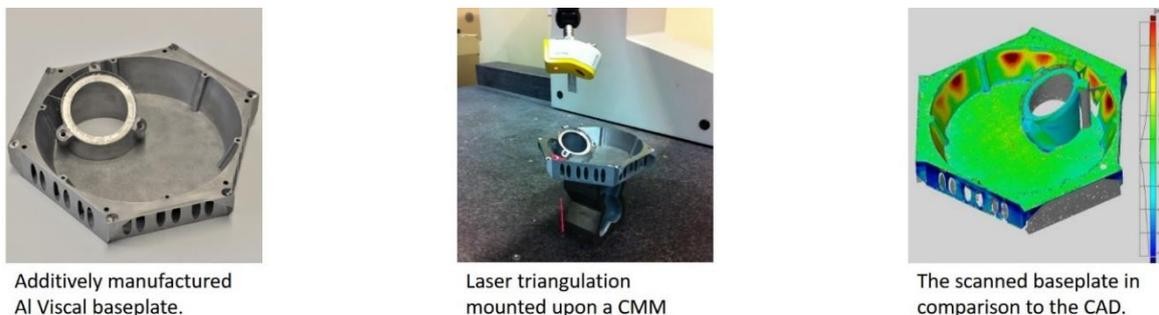
Figure 134: 3D scanning and comparison to the original CAD file of a Viscal base plate, image credits TNO.
