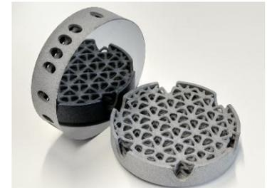
Optical mirror concept with internal lattice structure
