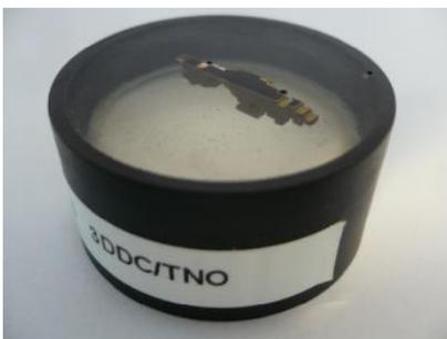
Copper Nickel Gold plated 3D Printed acrylic sample manufactured by Vat Photo Polymerisation.
