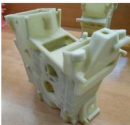
Wax model of the housing made by additive manufacturing.
