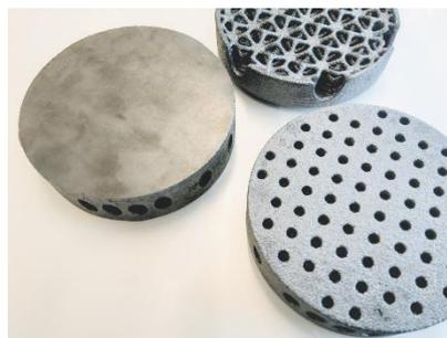
Si-SiC Mirror blanks printed by Binder Jetting technology. Produced by SGL Carbon
