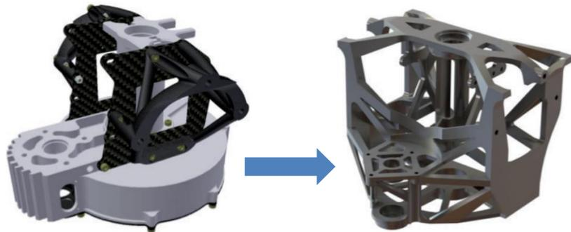
Material efficiency and lightweight structures in a 3D-printed helicopter frame for Flying Cam’s unmanned aerial vehicle (UAV), lowering the weight from 530 g to 392 g and thereby prolonging the drone’s battery life.
