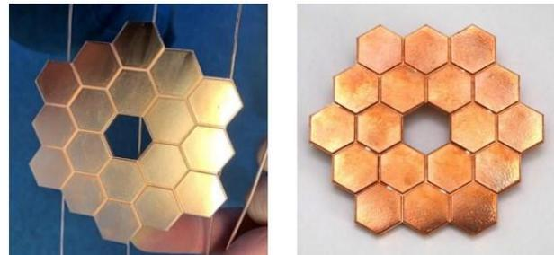
**Visual inspection** is used to ensure that a uniform metallic layer is plated, which is devoid of air bubbles.
