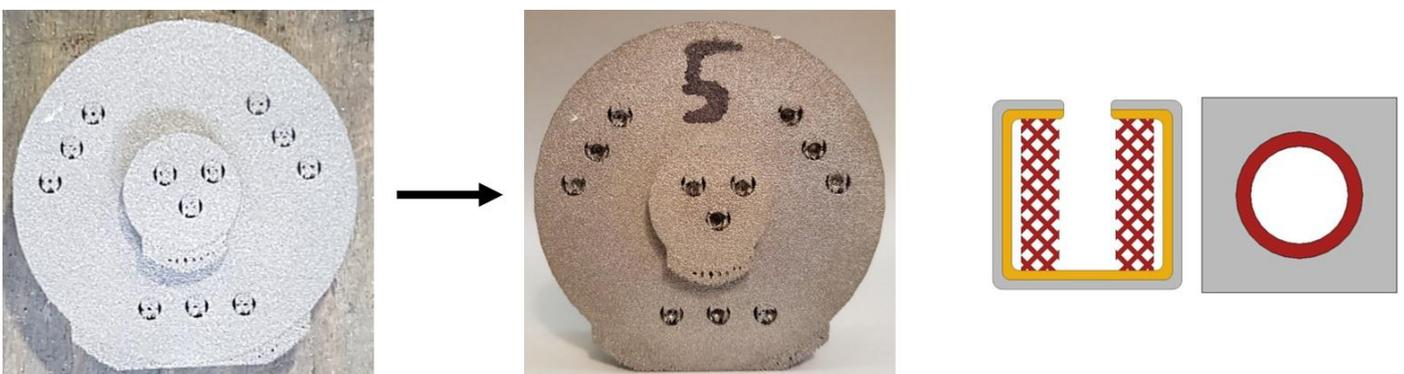
Figure 92: support removal problems; the example highlights the support material used to support the vertical circular holes and the failure at the support removal. Image credit: STFC & UoS.
