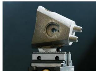
The handle is used to ease clamping. A 3d scan is made of the part positioned in the clamp.
