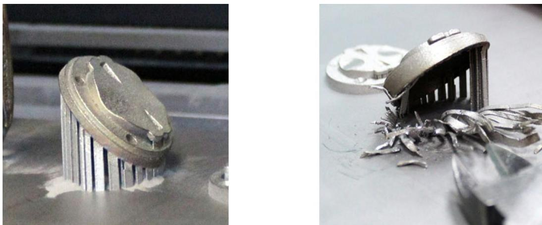
**Figure 88: removal of metal supports using cutting pliers, image credit: TNO.**
