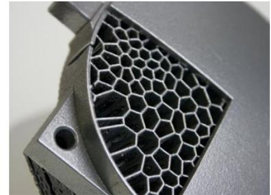
Additive manufactured mirror with internal structure made visible.
