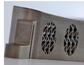
Oval holes to ease powder removal and to reduce weight
