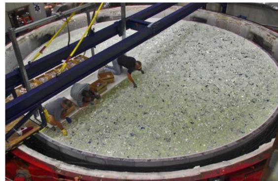
Figure 5: casting of lightweight mirrors. *Left* - sketch of the casting process, *right* - example of the casting of the GMT 8.4 m mirrors, image credit: H. M. Martin 2019 [5].
