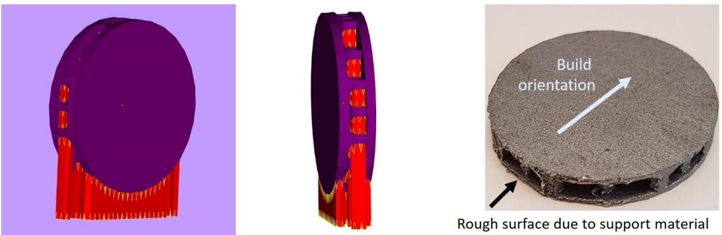
Figure 90: *left & middle* - support material generated for an aluminium L-PBF circular mirror substrate; *right* – roughness observed at the support – substrate interface, image credit CA Models & NSTP3-PF-007.
