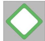
The circular holes have been converted into diamonds which are self supporting and do not require supports.
