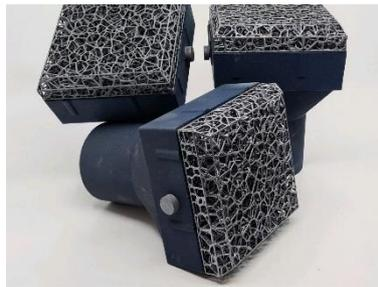
Silicon Carbide solar absorber based on
