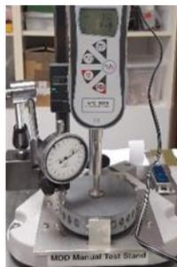
Test Bench for the TNO Sample in PA12
