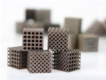
Low-density 3D lattice structures printed for the LIGHT additive manufacturing project consortium; (image credit: Delcam).
