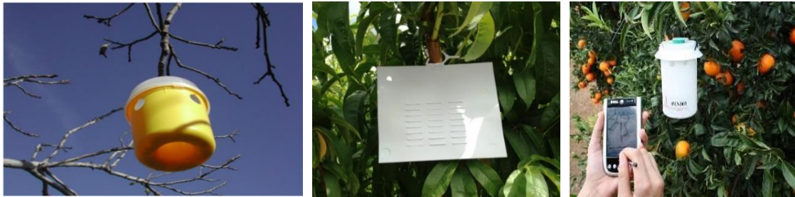
Figure 4.3.1 – Different types of traps used in Spain (left-Tephri-type traps, center- Magnet™ Med Trap and right- “Attract and Kill” trap) .
