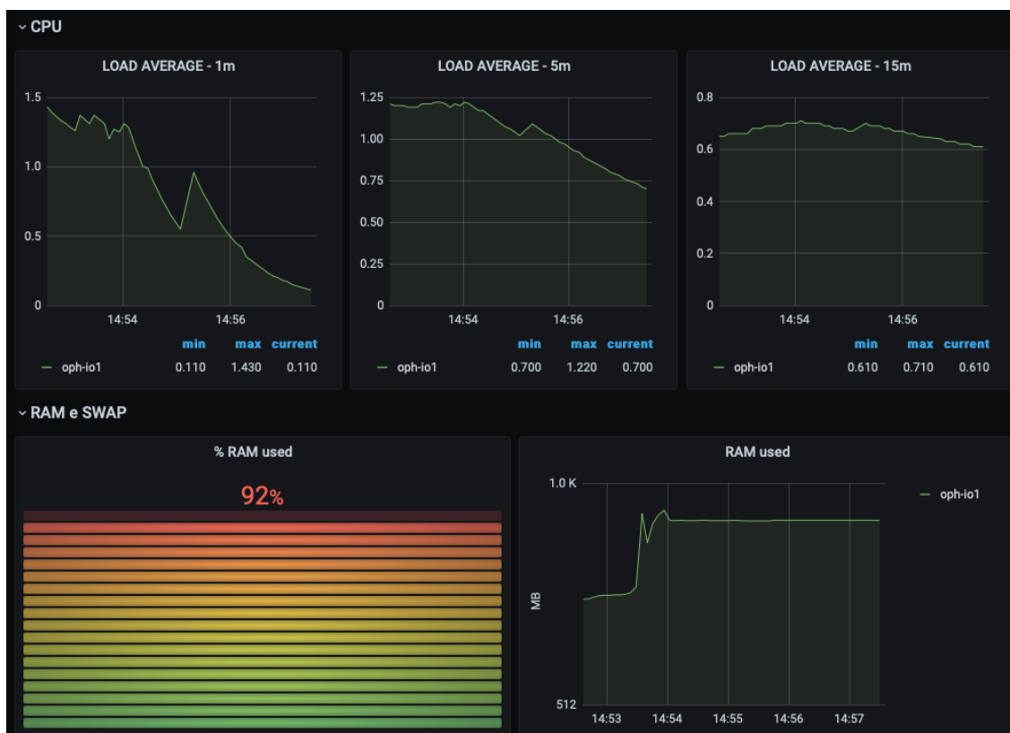
Figure 4.5: Infrastructure Metrics dashboard showing the monitoring metrics of the active working node
