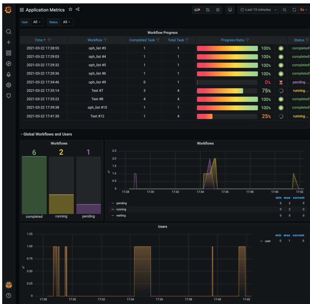
Figure 4.6: a section of the Application Metrics dashboard and, in particular, the workflow progress table and a panel visualizing information about the total number of workflows, grouped by status.
