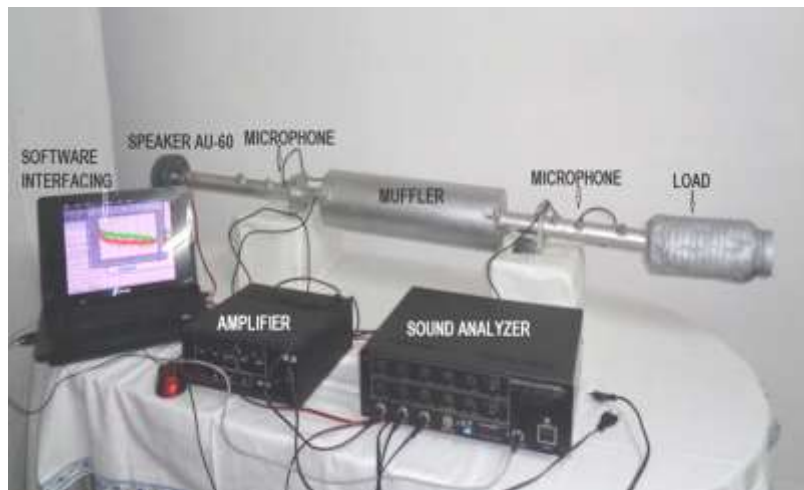
Figure 1: Muffler Transmission loss measurement setup with load
