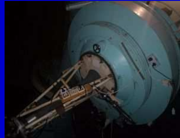
A-low resolution spectrograph R \sim 700 \lambda\lambda = 4200 - 7200 \text{ \AA}
