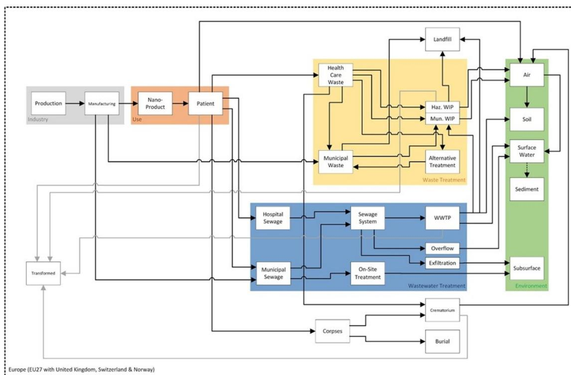
Figure 1: Structure of the material flow model used to track the NBMs through their lifecycle from production and manufacturing to their incorporation into medical products and then through to their elimination via waste and wastewater treatment until they finish in the environment. Figure taken from Ref. 1.
