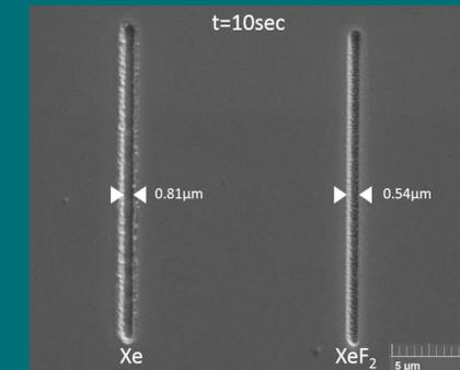
SEM image of trenches made using Xe (left) and XeF<sub>2</sub> (right) etching. Etching parameters were 30keV beam energy, 100pA beam current, and 10 sec etch time
