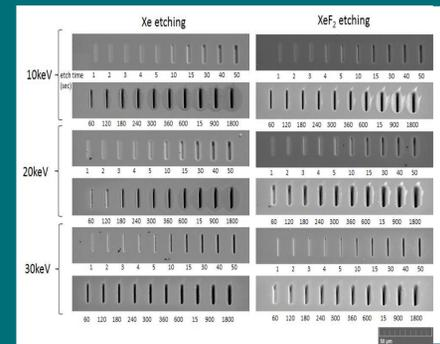
SEM images taken at a 55° angle of etches made using Xe plasma FIB milling with a beam energy of 10keV, 20keV, 30keV without (right) and with (left) fluorine gas injection.
