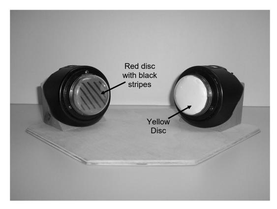
Figure 1. Apparatus with two microswitches (AbleNet Inc., model One-Step Communicator 20®) mounted and facing each other at a 90° angle, viewed from the participant's perspective. The distance between the microswitches was 12.5 cm. The yellow and red with black stripes colour discs could be changed across trials as needed.
