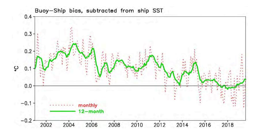
Monthly (dotted red) and 12-month running averaged (solid green) ship SST biases defined as the difference between ship and buoy SSTs.
