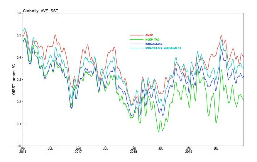
The light blue line represents the OISST using the new ship bias correction. It is more consistence with GMPE.
