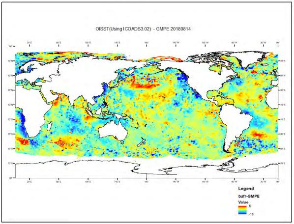
OISST anomaly relative to the GHRSST Multi-Product Ensemble (GMPE) for Aug. 14, 2018. The cold bias was very noticeable when OISST was run using in situ data from NCEP TAC only (left panel), and much smaller when run with data from ICOADS3.02(right panel)
