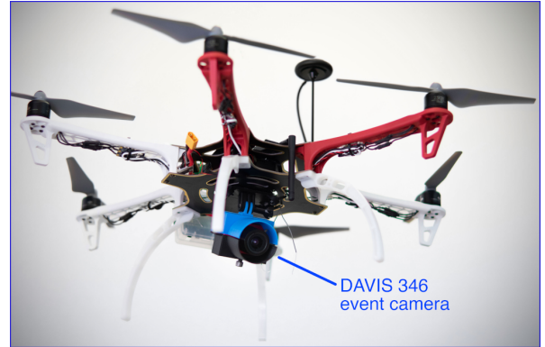
Fig. 6: The experimental platform: DJI Flamewheel F550 hexarotor equipped with an iniVation DAVIS346 camera.
