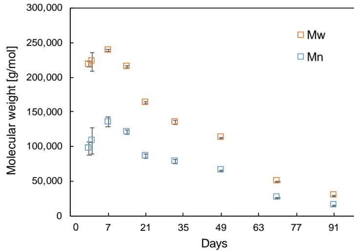
Figure 4 Evolution of number average molecular weight  $M_n$  and weight average molecular weight  $M_w$  over accelerated degradation period with error bars showing standard deviations.
