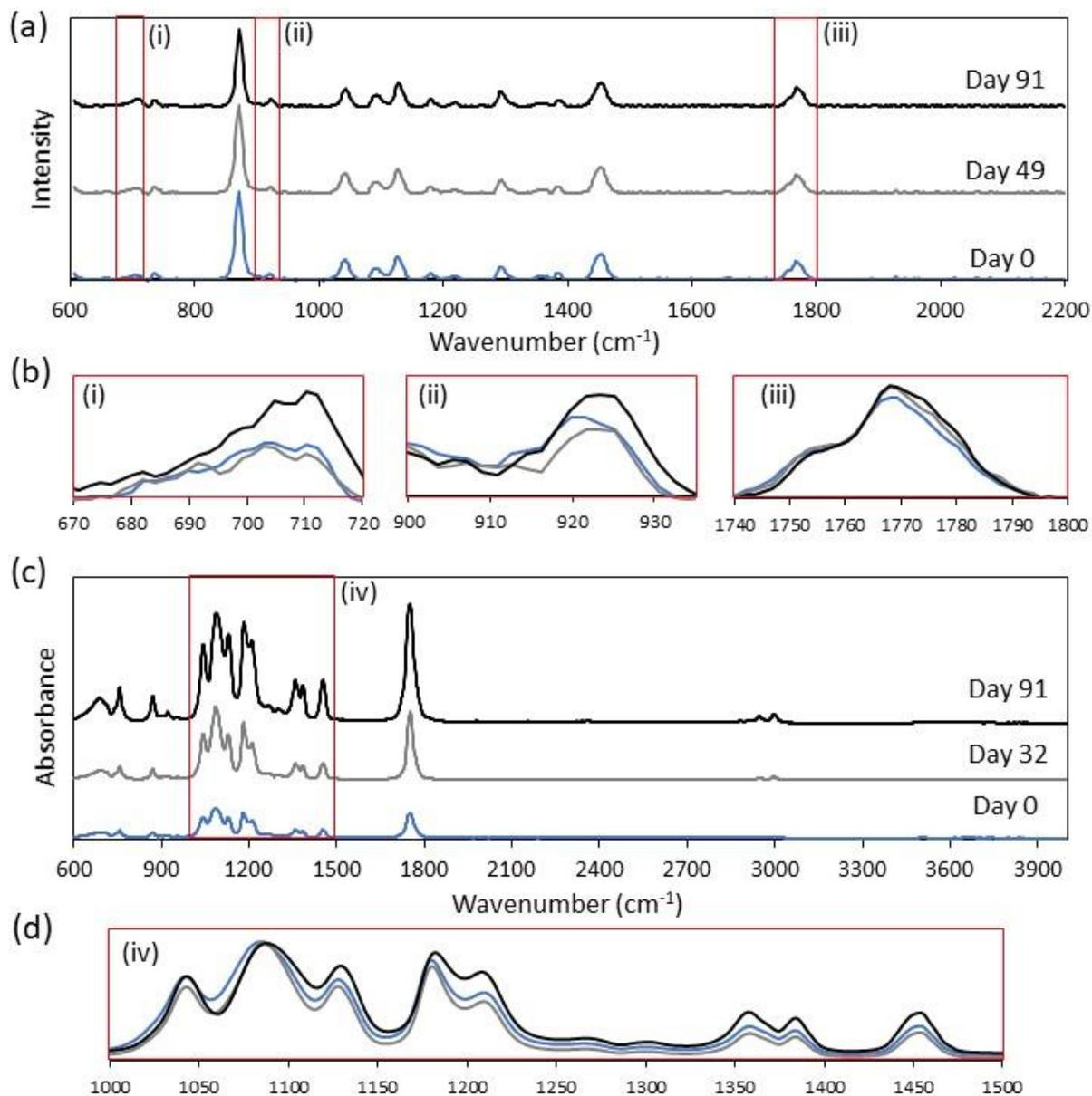
Figure 6 Raman spectra of PLLA samples from (a) 600  $\text{cm}^{-1}$  to 2200  $\text{cm}^{-1}$  (b) 670  $\text{cm}^{-1}$  to 1800  $\text{cm}^{-1}$  before, after 49 days and 91 days of accelerated degradation. Infrared spectra of PLLA samples from (c) 600  $\text{cm}^{-1}$  to 4000  $\text{cm}^{-1}$  (d) 1000  $\text{cm}^{-1}$  to 1500  $\text{cm}^{-1}$  before, after 32 days and 91 days of accelerated degradation.
