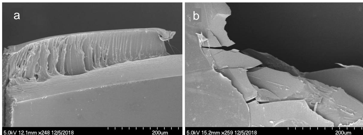
Figure 7 SEM images of dog-bone samples damage surfaces obtained with 5kV and magnification approximately x250. (a) Failure surface of a dog-bone sample before degradation exhibiting ductile failure in tensile test. (b) Failure surface of a dog-bone sample after 112 days of degradation showing brittle fracture resulting from gentle handling.
