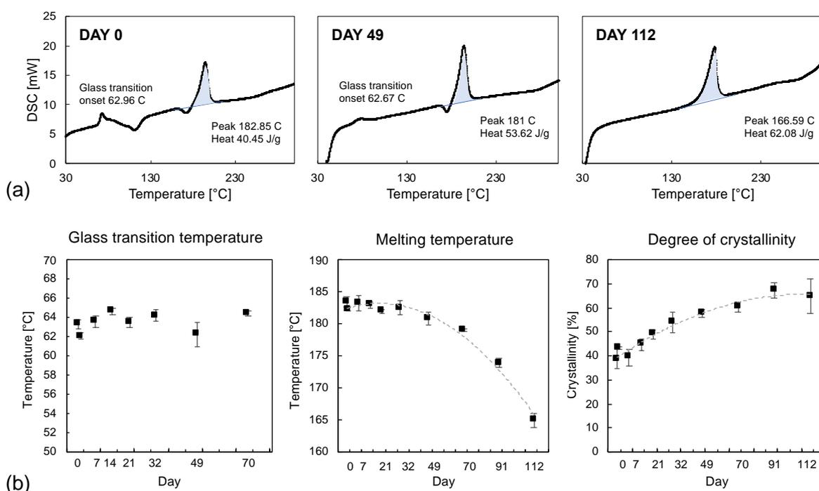
Figure 5 (a) DSC signal in PLLA samples before, after 49 days and 112 days of accelerated degradation. (b) Glass transition, melting point and degree of crystallinity evolution of PLLA samples during accelerated degradation.
