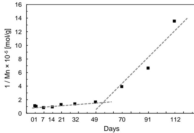
Figure 9 Degradation rate  $1/M_n$  versus time showing distinct rate increase on day 52 of accelerated degradation of PLLA.
