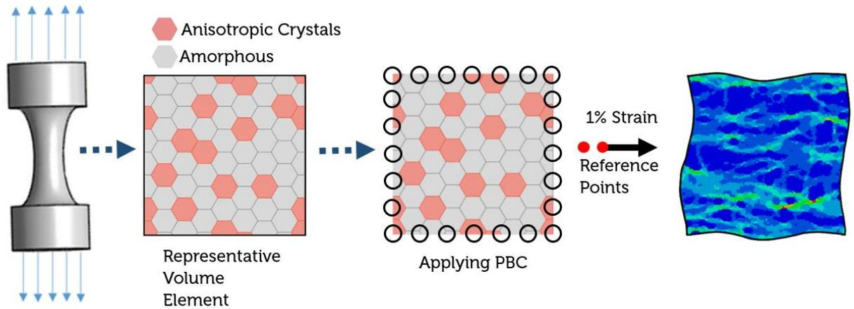
Figure 2: Micromechanical modelling of a semi-crystalline polymer using a representative volume element (RVE) approach.
