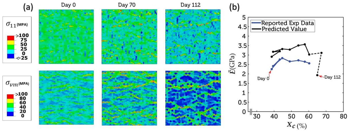
Figure 10 Results from micromechanical simulations. (a)  $\sigma_{11}$  and  $\sigma_{vm}$  distribution at three selected time points. (b) Model predictions (black) compared to experimental data.
