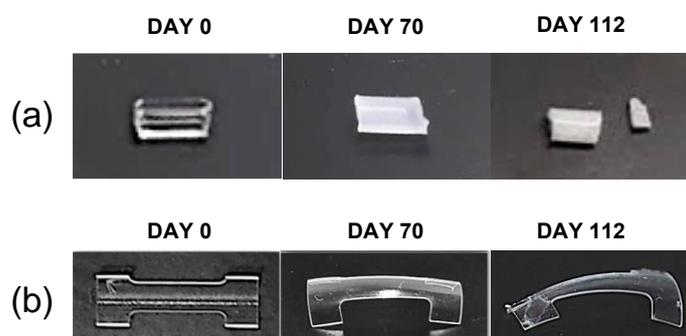
Figure 3: (a) Tubular samples used for mass change, GPC and DSC experiments changed from transparent to opaque and brittle with degradation. (b) Dog-bone samples used for tensile testing deforming during degradation.
