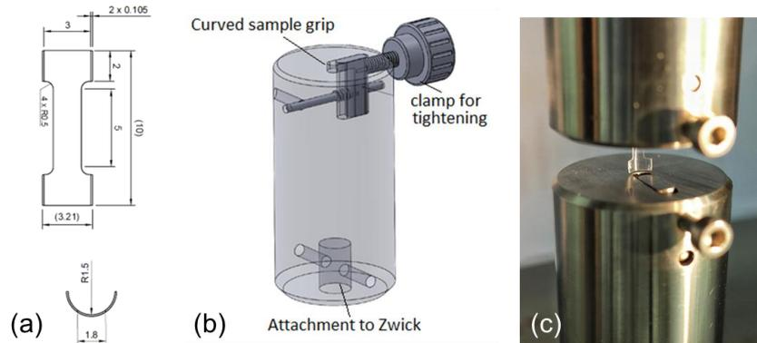
Figure 1 (a) Shape and dimensions of the samples used in the accelerated degradation study. (b) Dedicated clamps designed to grip curved shaped dog-bone samples. (c) Clamps with dog-bone sample being inserted.
