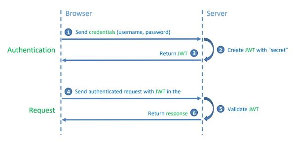
Figure 3: Securely transmitting information between parties with JWT.
