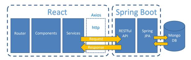
Figure 4: Architectural Design Diagram.
