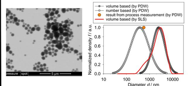
Electron microscope image of synthesized polyvinyl acetate particles (left) and particle size distributions from PDW spectroscopy and static light scattering (right).
