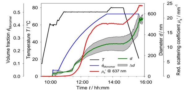
Temperature  $T$ , monomer volume fraction  $\phi$ , reduced scattering coefficient  $\mu'_s$  at 637 nm, mean diameter  $d$  and its distribution width  $\Delta d$  as function of time  $t$  for the polymerization of vinyl acetate.
