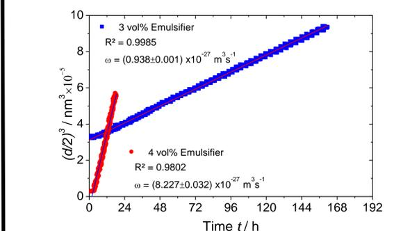
Cubic nanodroplet radius as function of time for two different emulsifier concentrations (points) and linear fit (lines) to obtain the according Ostwald ripening rates  $\omega$ .
