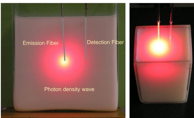
Spherical PDWs in dispersions of polymer nanoparticles.
