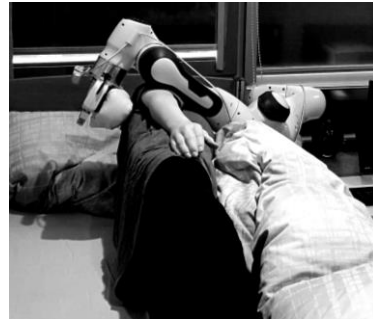
Figure 3: Robot holding a patient simulator
