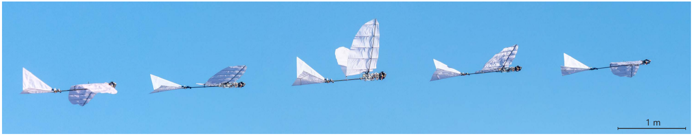
Figure 12. Composite image of the E-Flap along a flapping cycle during outdoor flight.
