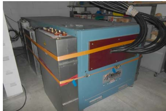
Fig.15 Main capacitor block (blue casing) and 3 external capacitors added on each side of the main device.
