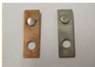
Fig. 1 Stationary (right) and movable (left) electrodes in this study.
