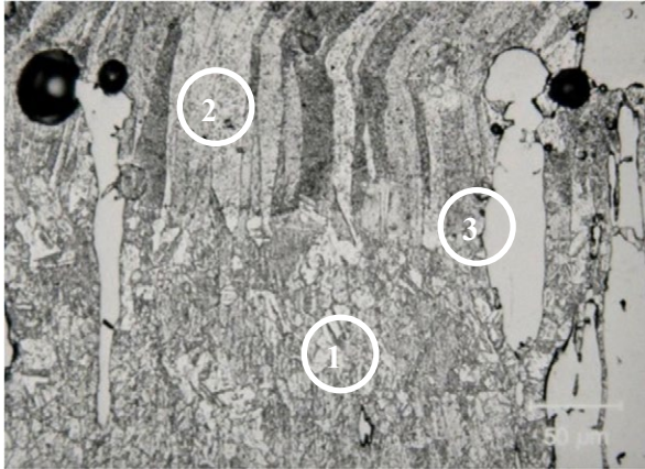
Fig. 2 Microsection of Ag/Ni 10 \perp after model switch test [11], for details refer to the text.
