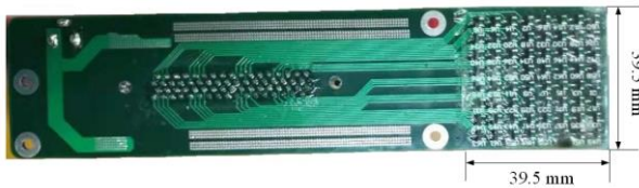
Fig. 3 Texas Instruments DRV5035-VA Hall-effect magnetic sensor array mounted on PCB.
