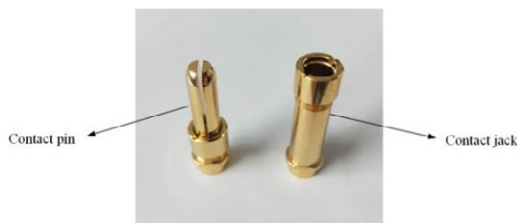
Fig. 1 The contacts specimen of electrical connector
