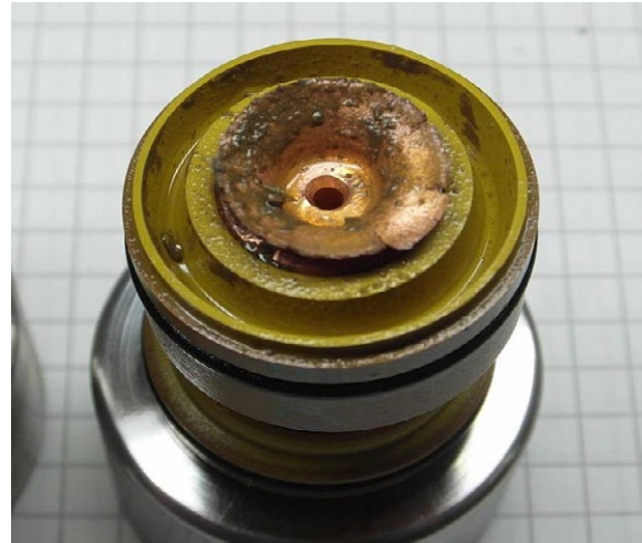
Fig.23 Separated tube part 1 of Fig.21 after ignition and delaboration, photographed more inclined; no copper particle is broken!
