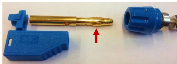
Fig. 5 Banana plug connector with an integrated contact spring in the male plug (arrow). It provides a multi-contacting in the cylindrical female connector at the right hand side.
