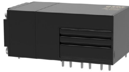
Fig. 9 Prototype of fast switching device to change between 380 VDC and 270 VAC supplies (continuous operating current 16 A DC, 20 A AC).
