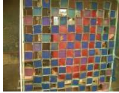
Fig. 7 View of the arc flash indicators used for the test
