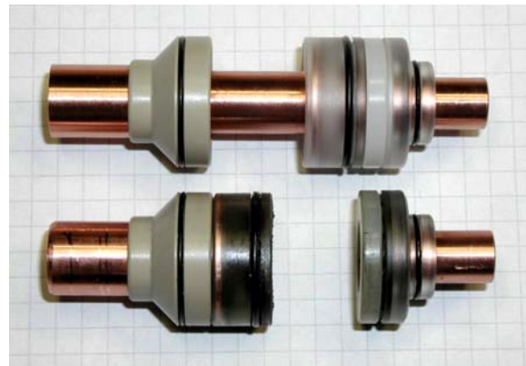
Fig.19 The switching tube made of copper before (above) and after triggering the internal EED (below); the folding area ist completely covered by isolator and sabot.
