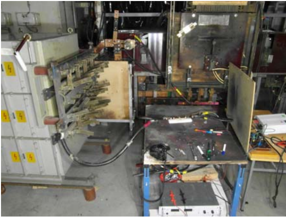
Fig.16 The work bench of the AIT laboratory. Left the resistor and inductance device, middle behind the connectors of the trafostation and middle in front the work table.
