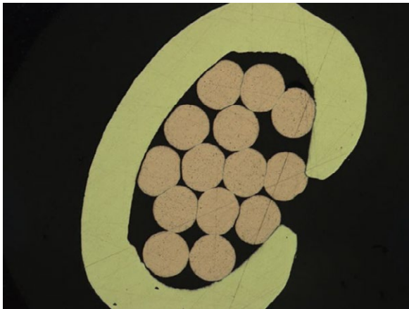
Fig. 12 Insufficient crimping. Image: Courtesy of RoodMicrotec
