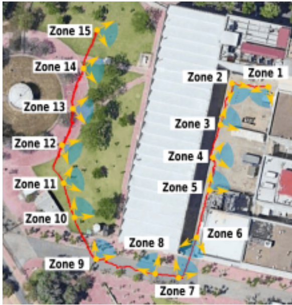
FIGURE 6: Example of surveillance mission used in the system experimentation conducted at the laboratories of the School of Engineering of the University of Seville. The frames represent the 6 DoF waypoints in the surveillance mission. The blue circular sectors represent the field of view of the event camera at each waypoint.
