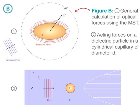
**Figure B:** ① General calculation of optical forces using the MST. ② Acting forces on a dielectric particle in a cylindrical capillary of diameter d.
