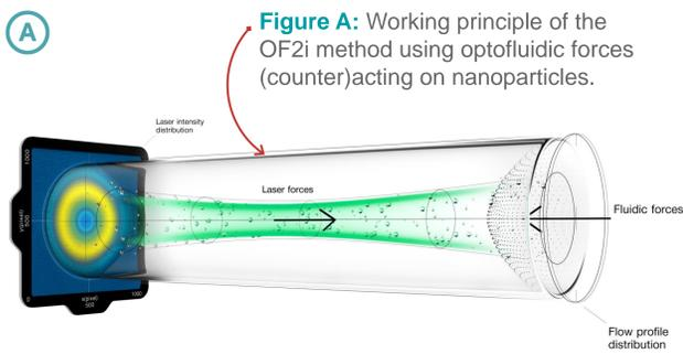
**Figure A:** Working principle of the OF2i method using optofluidic forces (counter)acting on nanoparticles.
