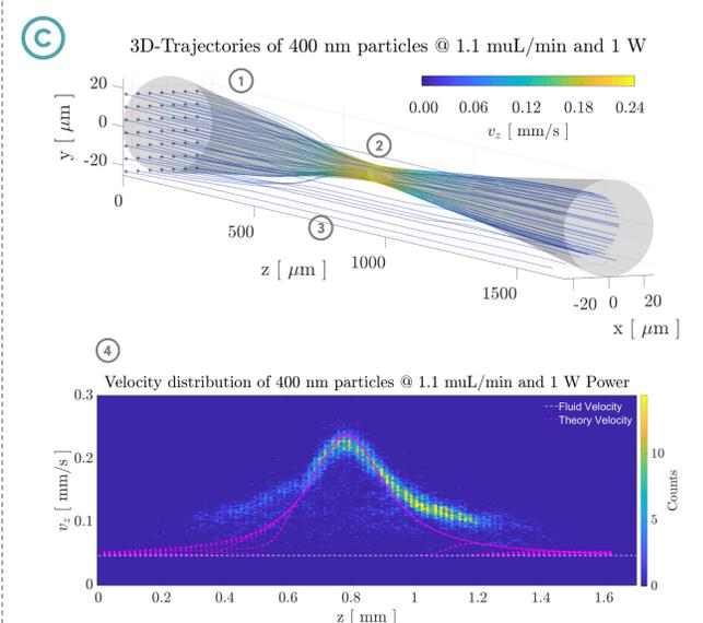
**Figure C:** ① - ③ Simulated trajectories of standardized Latex-particles with diameters of 400 nm where optical and fluidic forces act in the same direction. ④ Theoretical calculations and experimental data (histogram) of single particle trajectories.
