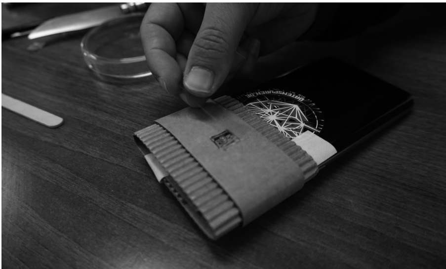
Fig. 1: A participant demonstrates the assembly of their DIY cardboard microscope. A clear piece of plastic cup would be used as sample holder in front of the lens.
