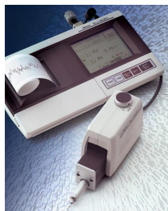
Fig. 4. The surface roughness tester Mitutoyo Surflest SJ-400
