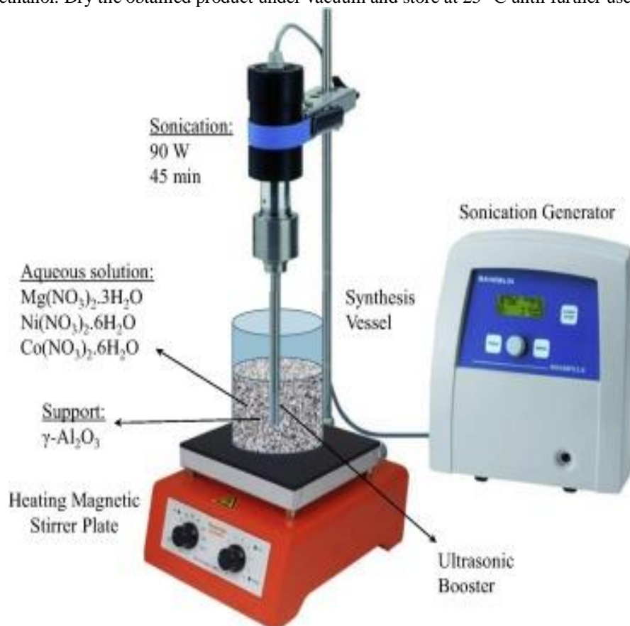
Figure 2 Ultra sound assisted synthesis
