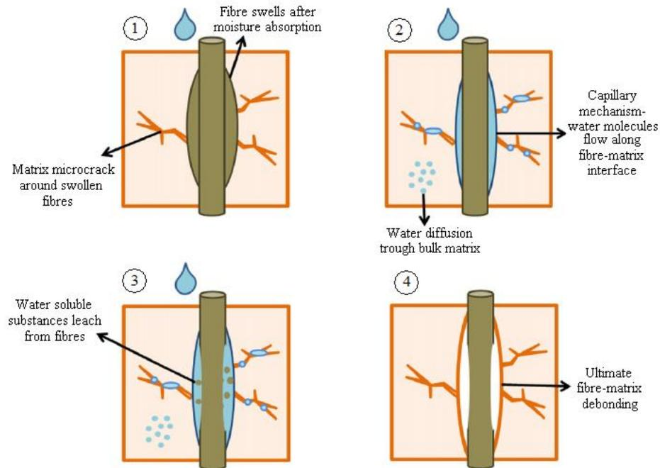
Figure 1.2. Debonding phenomenon between fiber and matrix – Adapted from [24].
