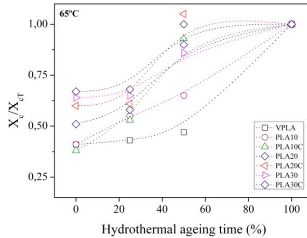
Figure 3.16. Plots of  $X_c/X_{cs}$  against % saturation for PLA and composites for 65 °C hydrothermal condition.
