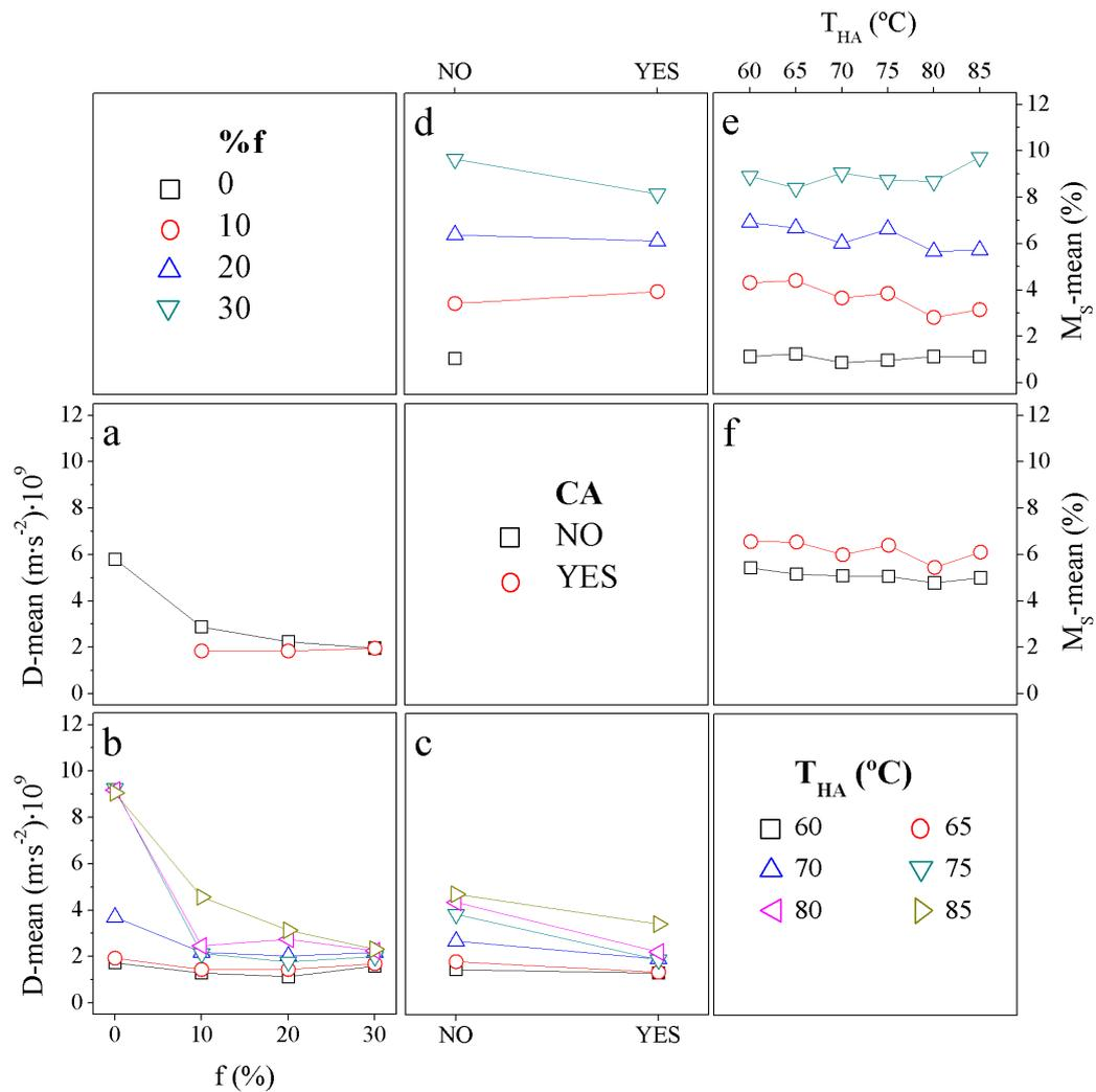
Figure 3.5. Interaction plot of  $M_s$  and  $D$ -means versus amount of fiber, coupling agent and temperature.
