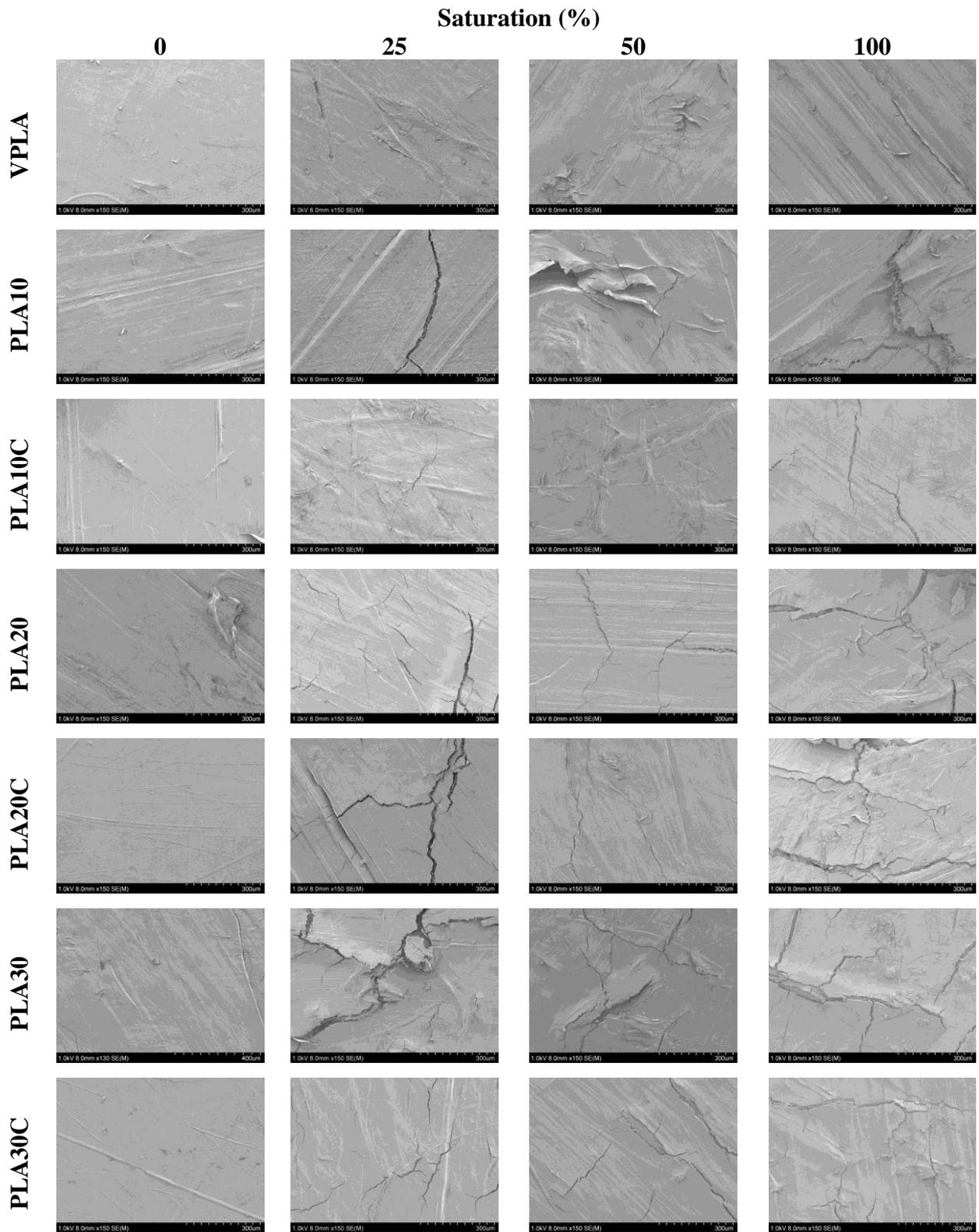
Figure 3.23. Micrographs for VPLA and composites at 85 °C for different saturation degrees.
