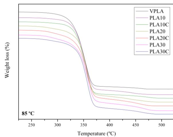
Figure 3.10. TG curves for VPLA and composites for 85 °C hydrothermal condition.
