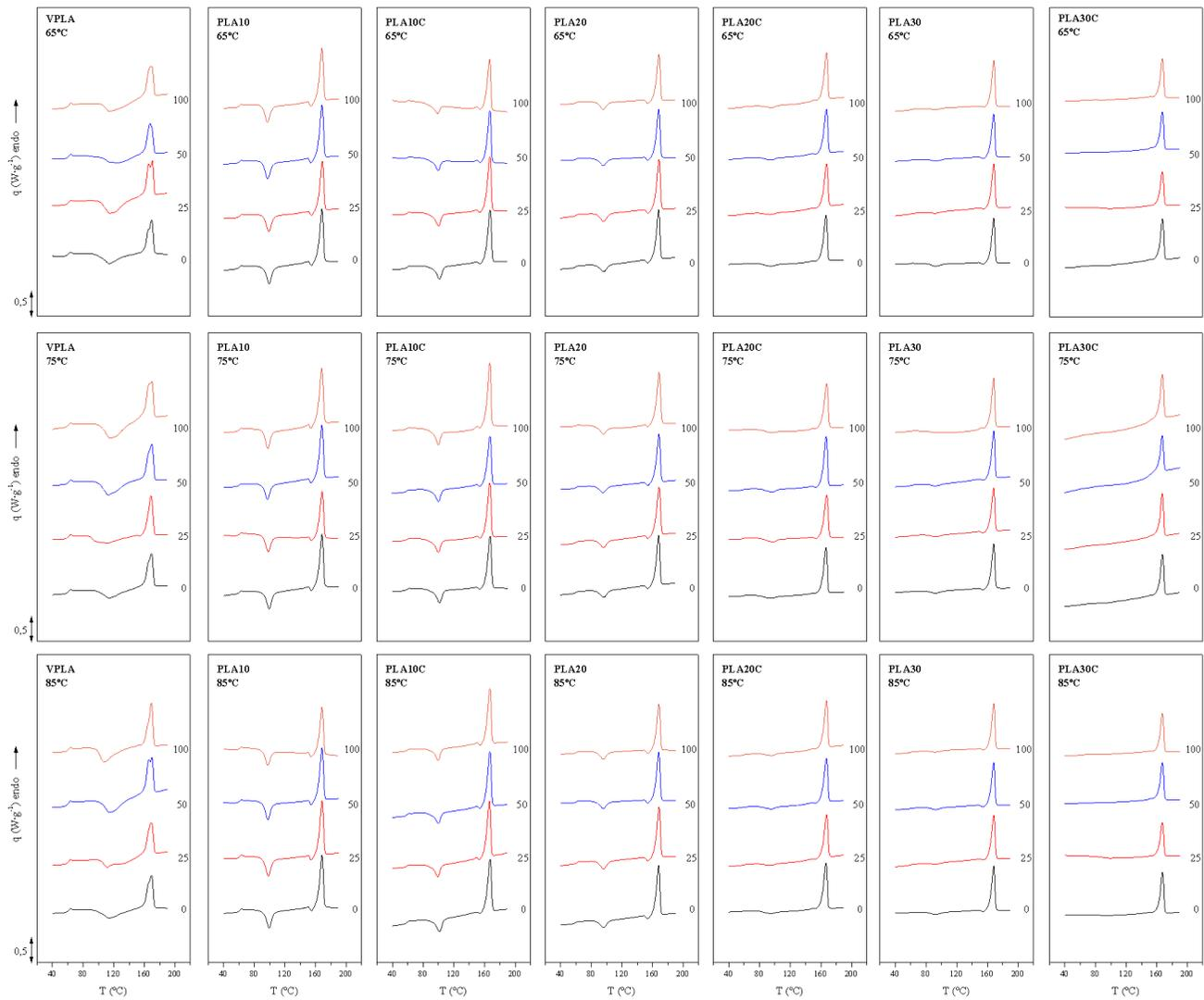
Figure 3.20. Second heating scan for PLA and composites for different hydrothermal condition (65, 75 and 85 °C) and saturation degrees (0, 25, 50 and 100%).
