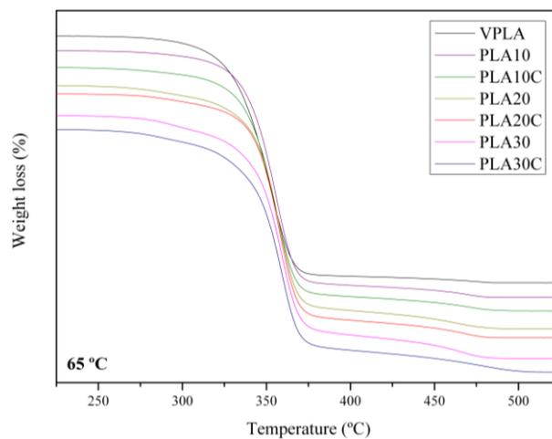
Figure 3.8. TG curves for VPLA and composites for 65 °C hydrothermal condition.
