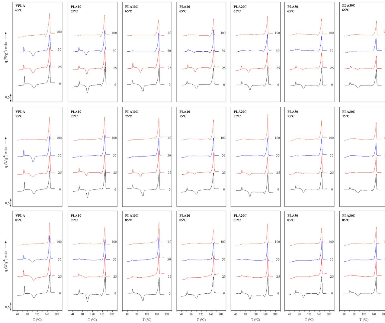
Figure 3.15. First heating scan for PLA and composites for different hydrothermal condition (65, 75 and 85 °C) and saturation degrees (0, 25, 50 and 100%).
