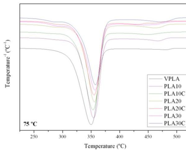
Figure 3.12. DTG curves for VPLA and composites for 75 °C hydrothermal condition.
