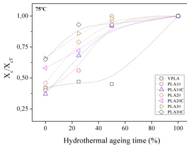
Figure 3.17. Plots of  $X_c/X_{cs}$  against % saturation for PLA and composites for 75 °C hydrothermal condition.
