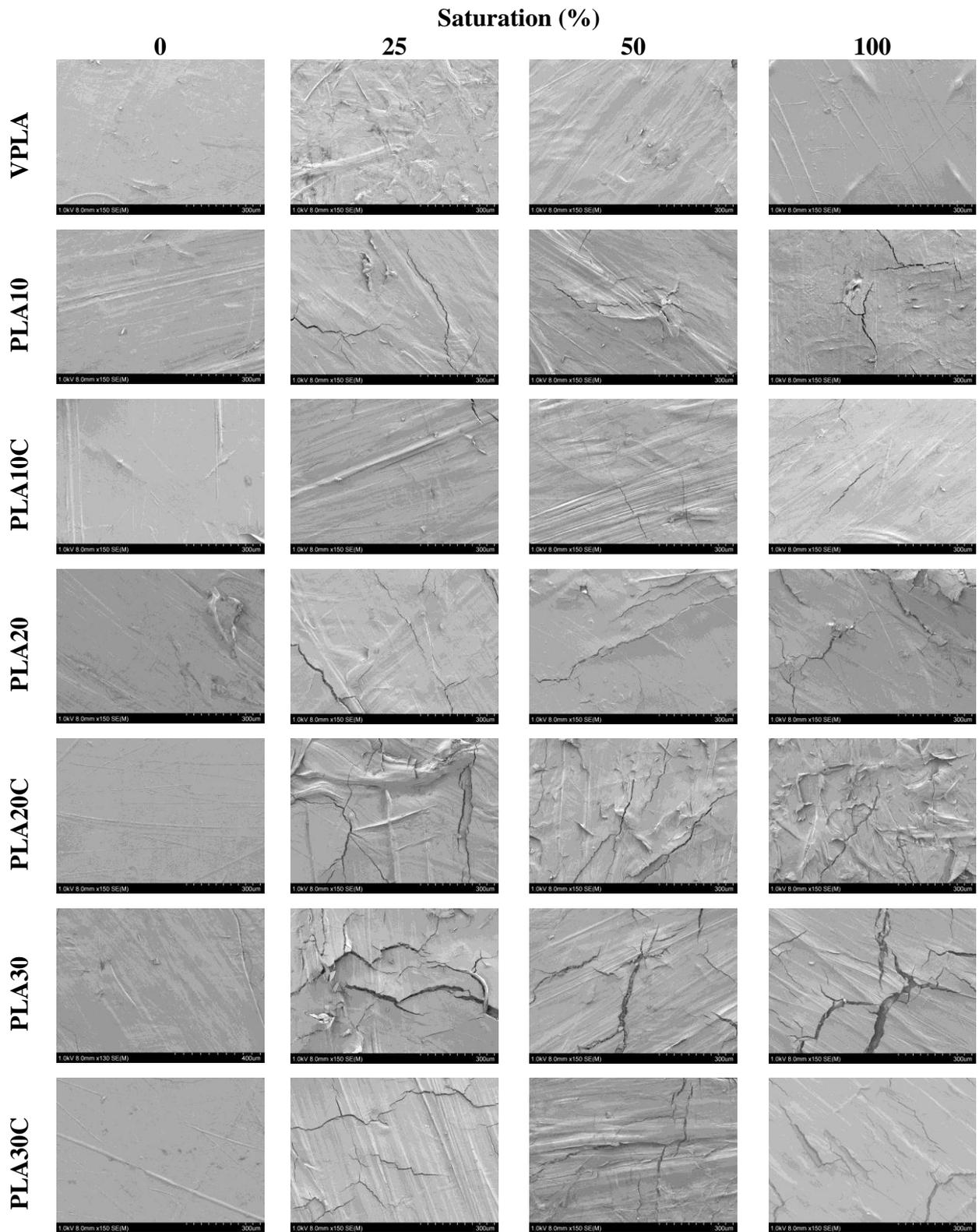
Figure 3.22. Micrographs for VPLA and composites at 75 °C for different saturation degrees.
