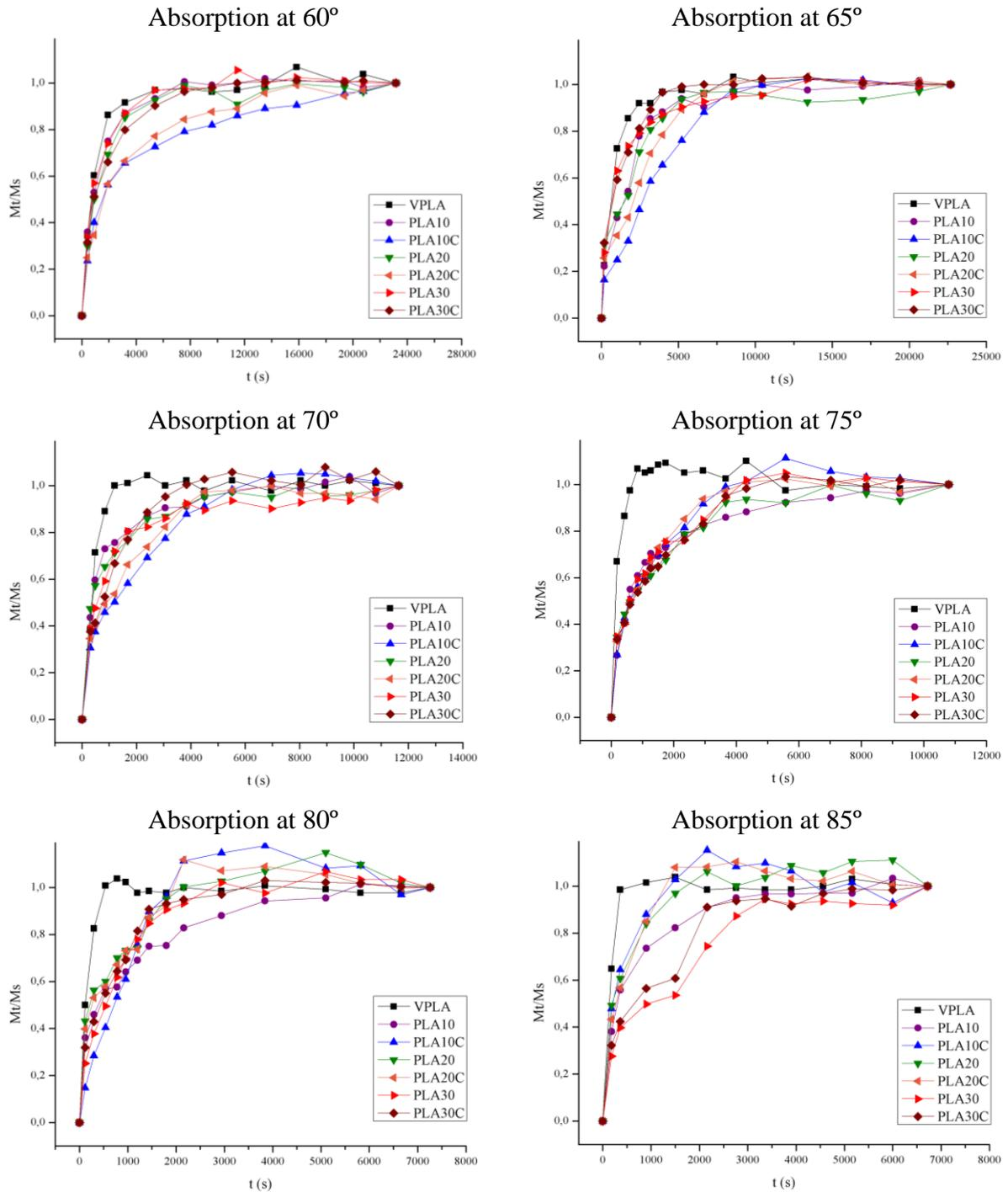
Figure 3.3. Plots of  $M_t/M_s$  against  $t$  for PLA and composites for all hydrothermal conditions.
