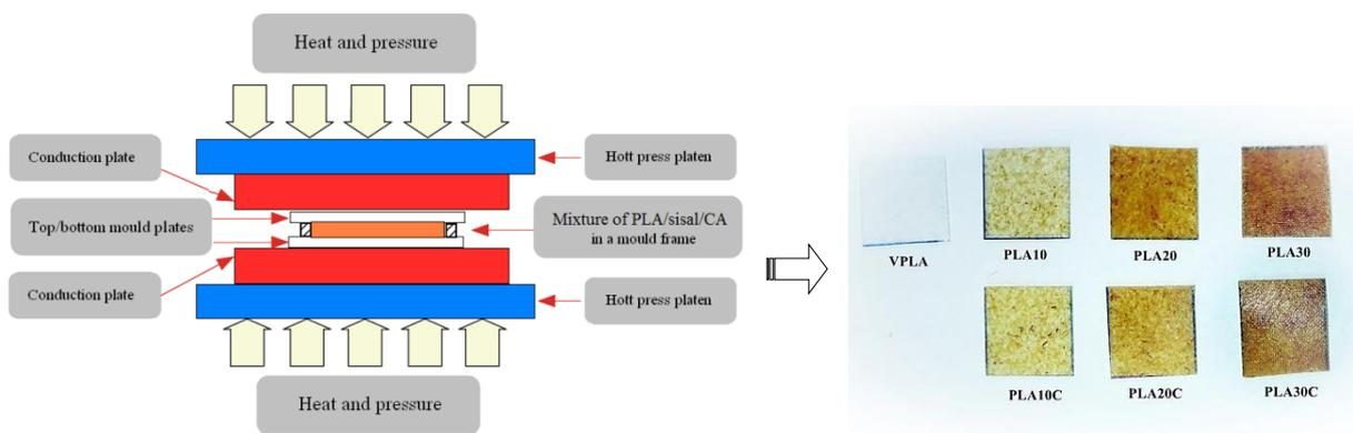
Figure 2.1. Compression moulding scheme –adapted from [24]– and PLA/sisal biocomposites sheets.
