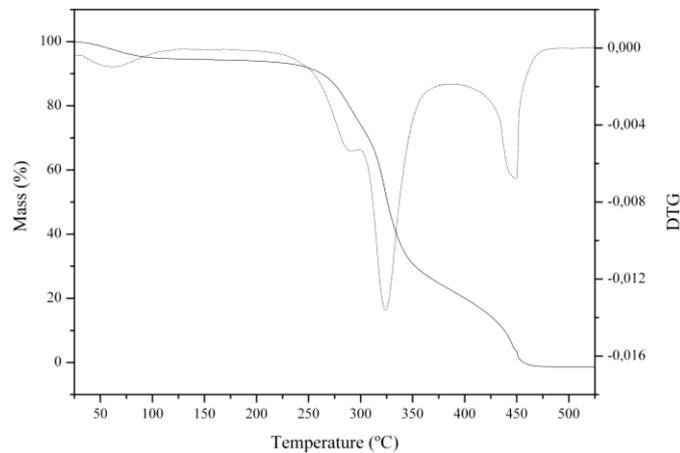
Figure 3.6. TG and DTG of untreated sisal fiber.
