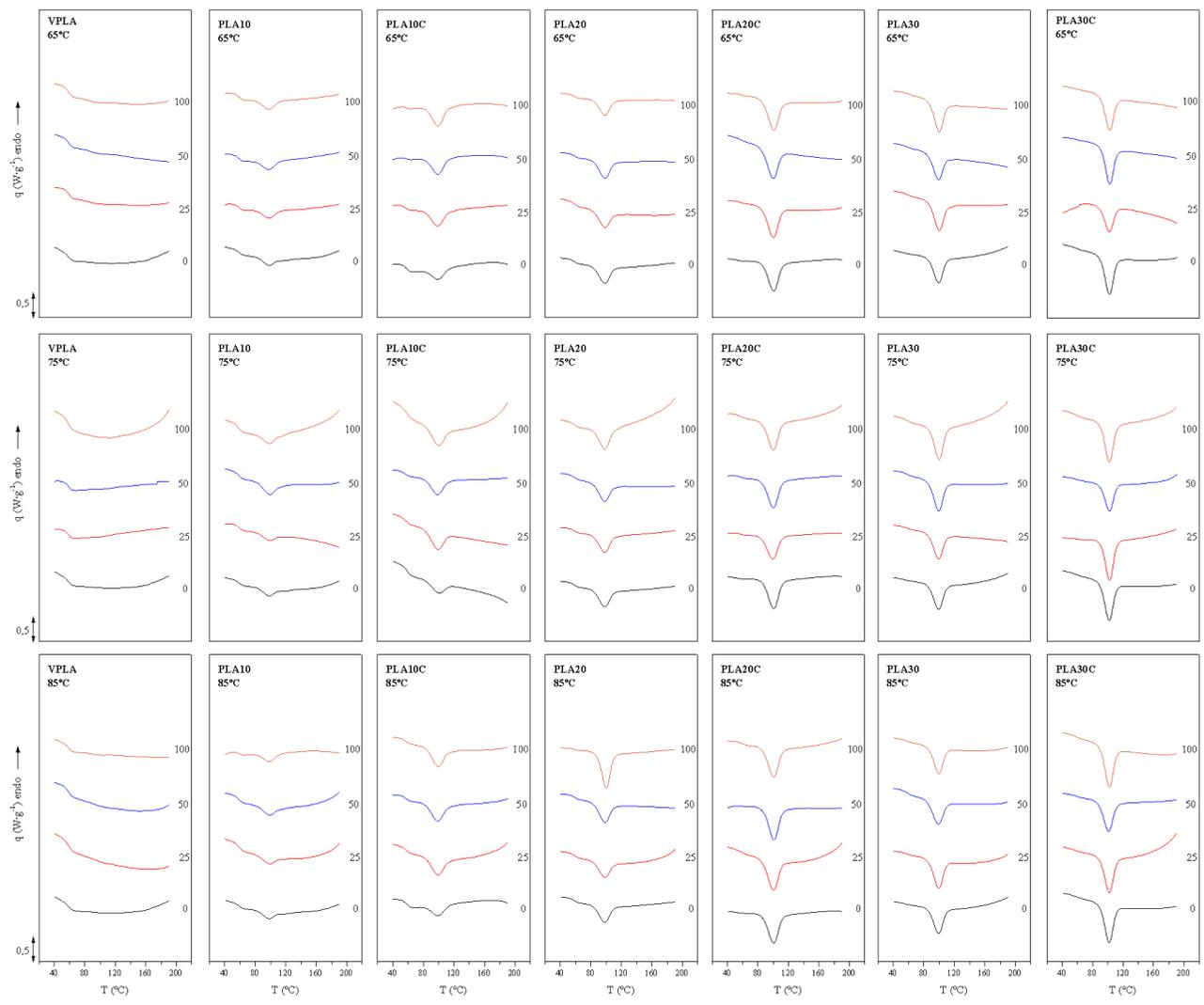
Figure 3.19. Cooling scan for PLA and composites for different hydrothermal condition (65, 75 and 85 °C) and saturation degrees (0, 25, 50 and 100%).
