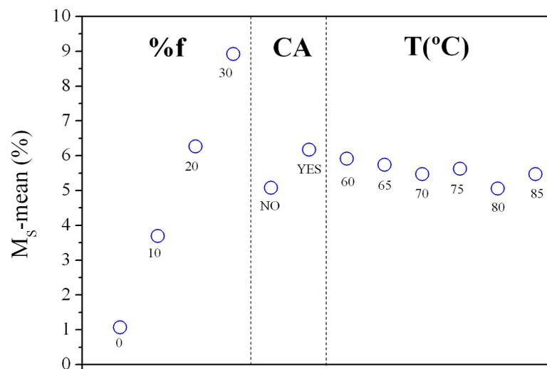
Figure 3.2. Plot of  $M_s$ -means versus fiber content, coupling agent and temperature.
