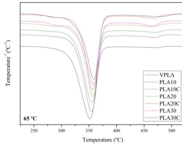
Figure 3.11. DTG curves for VPLA and composites 65 °C hydrothermal condition.
