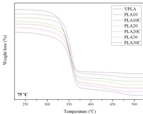
Figure 3.9. TG curves for VPLA and composites for 75 °C hydrothermal condition.
