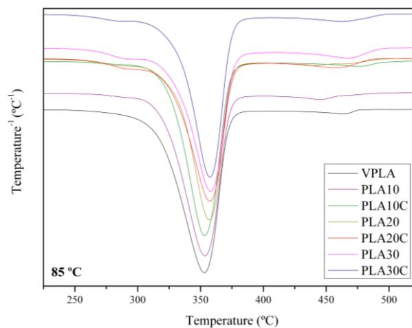
Figure 3.13. DTG curves for VPLA and composites for 85 °C hydrothermal condition.
