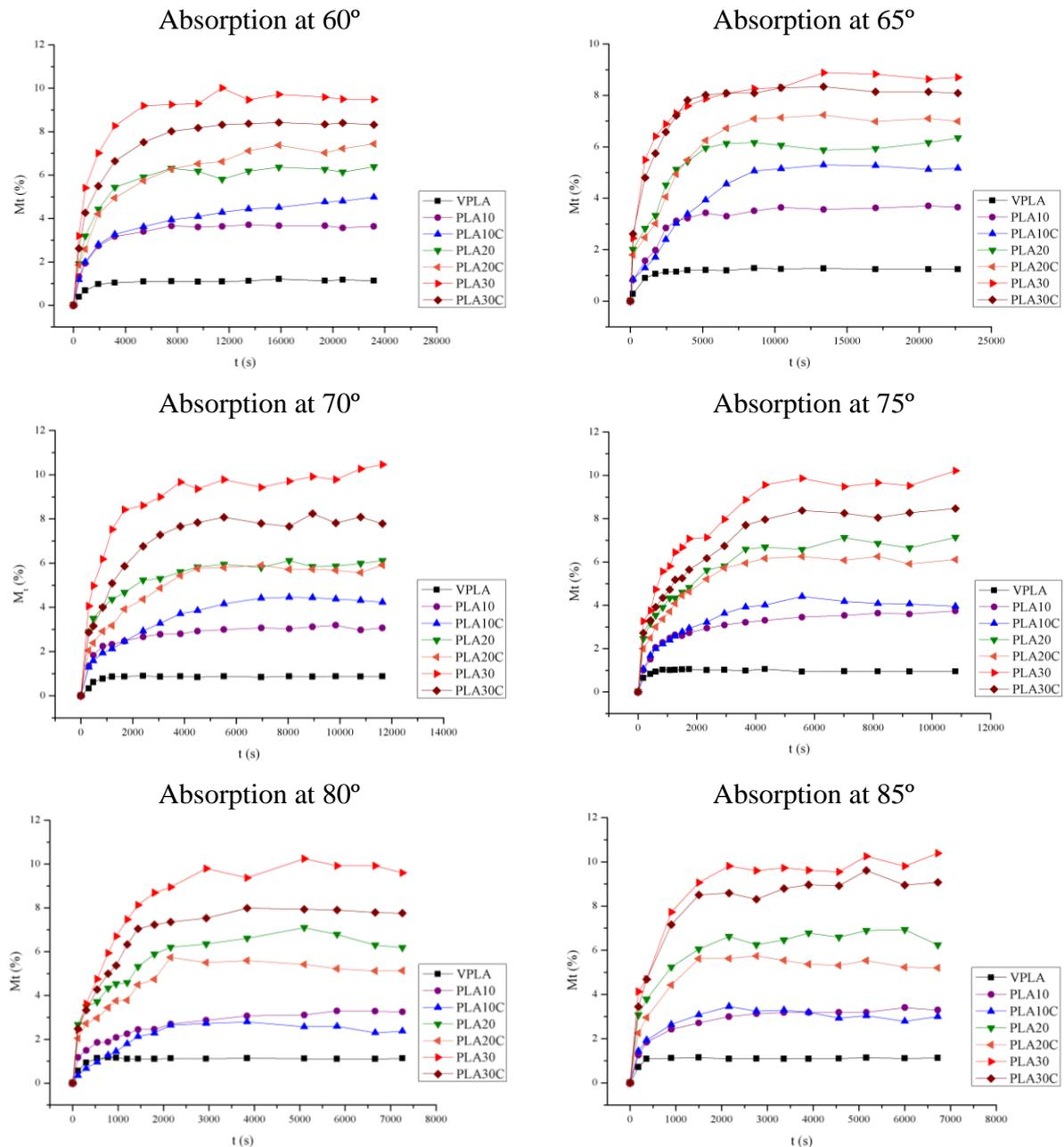
Figure 3.1. Plots of  $M_t$  against  $t$  for PLA and composites for all hydrothermal conditions.
