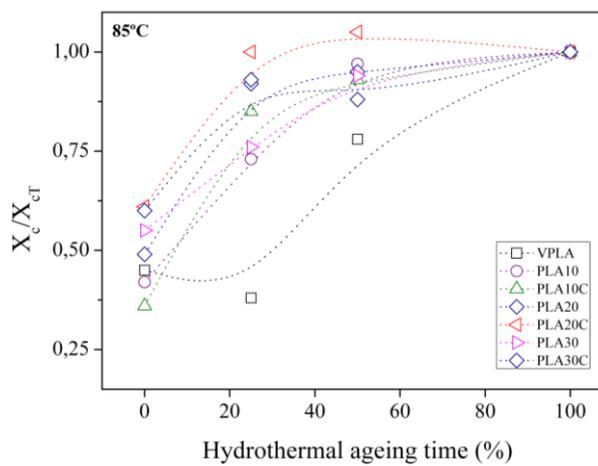
Figure 3.18. Plots of  $X_c/X_{cs}$  against % saturation for PLA and composites for 85 °C hydrothermal condition.
