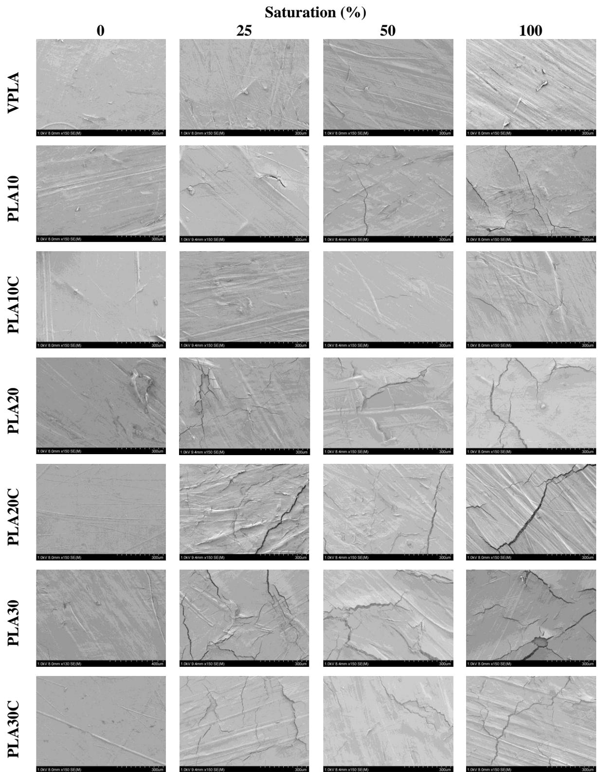
Figure 3.21. Micrographs for VPLA and composites at 65 °C for different saturation degrees.
