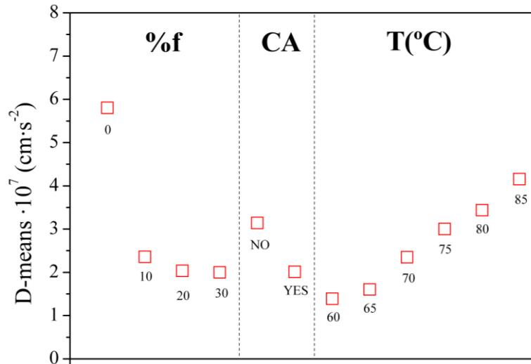
Figure 3.4. Plot of  $D$ -means versus fiber content, coupling agent and temperature.
