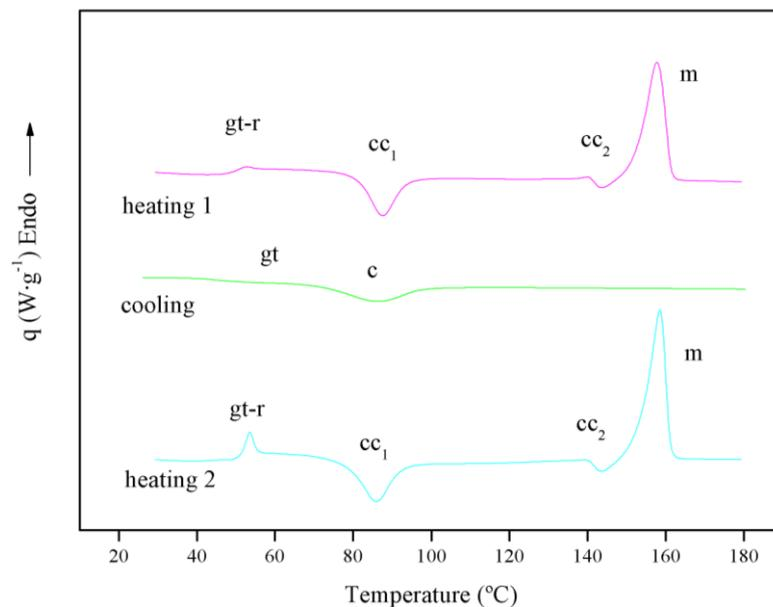
Figure 3.14. Example of events at first and second heating scan as well as cooling ramp.
