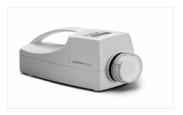
Pictured: Air sampling device used to take samples of hen houses for microbial analysis and detection of Campylobacter.
