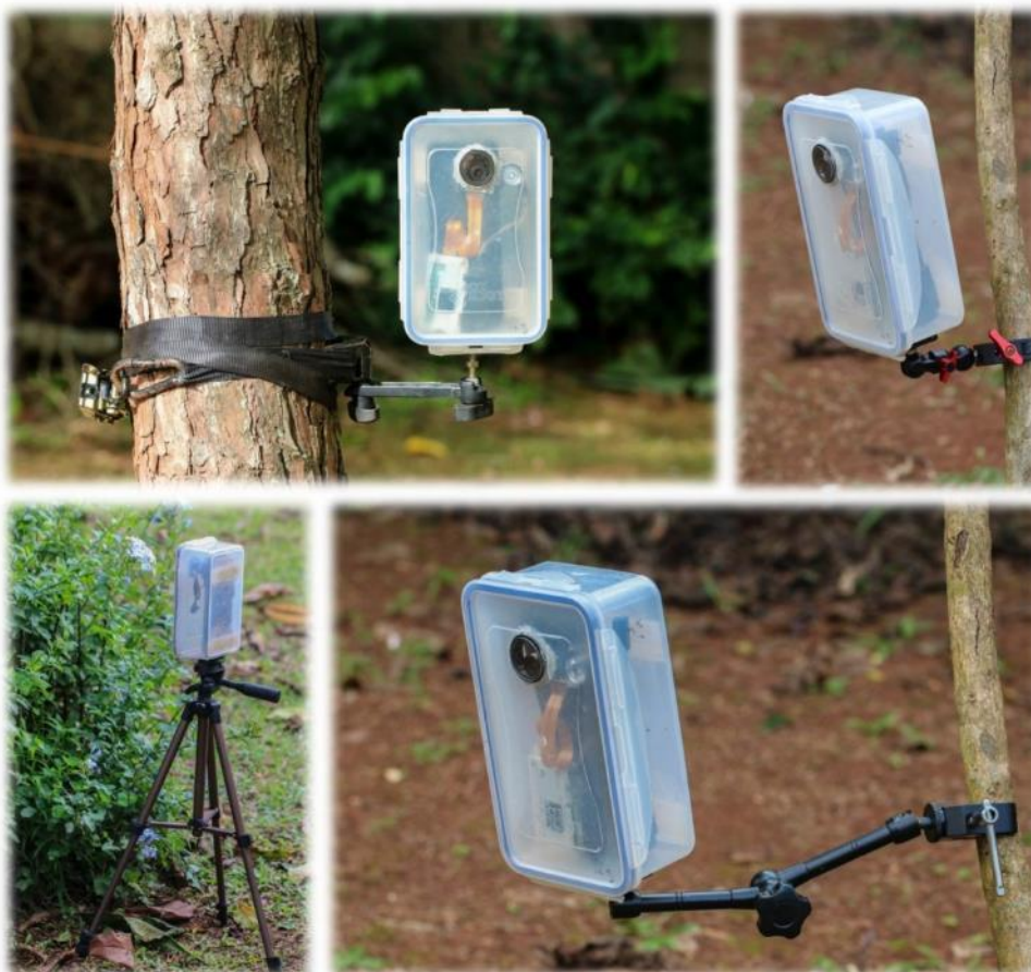
Figure 4. Example of various camera mounts that we successfully tested in the field.
