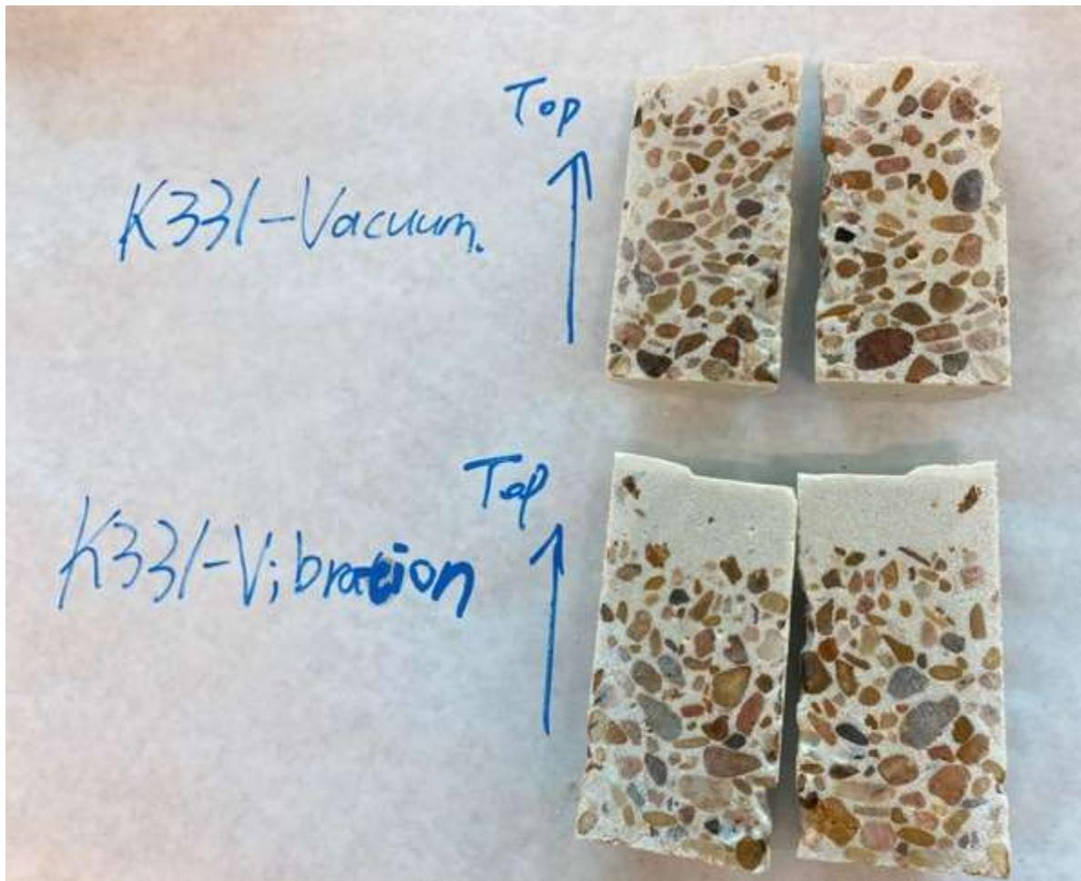
Figure 5. Different Ways to Minimize Porosity in GPC Concrete.
