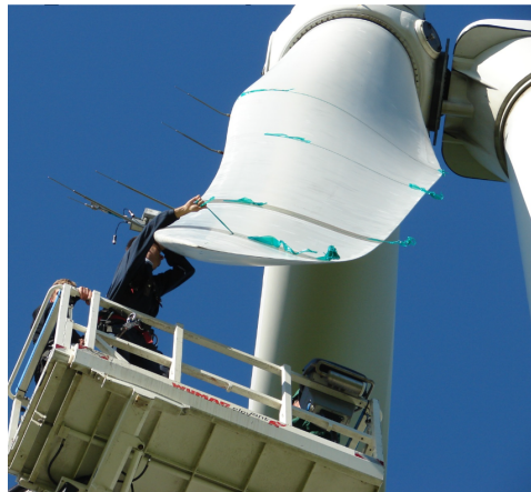
Figure: Installation of measurement system of DANAERO - DTU Wind Energy
