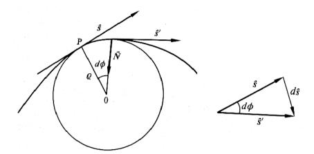
The inverse of the radius of curvature is the magnitude of the first derivative of the tangent vector, or the second derivative of the position vector.
