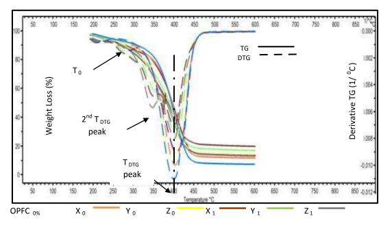
Figure 1: Thermogravimetric analysis (TGA) and derivative of thermogravimetric (DTG) curves of various flame retardant formulations in OPFC panel
