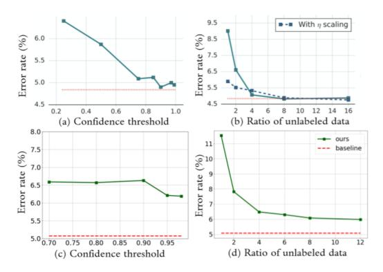
**Figure 1**. Plots of various ablation studies on FixMatch compared with those reported in the paper. (a) Varying the confidence threshold for pseudo-labels in the original paper. (b) Varying the ratio of unlabled data ( $\mu$ ) in the original paper. (c)Varying the confidence threshold for pseudo-labels based on our implementation. (d) Varying the ratio of unlabled data ( $\mu$ ) based on our implementation.
