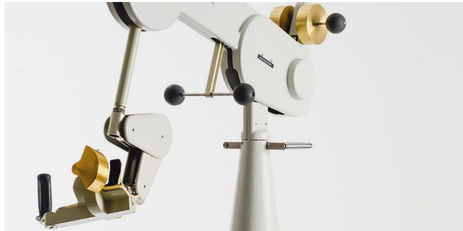
Figure 1. The body of the passive robotic arm called Track-Hold.
