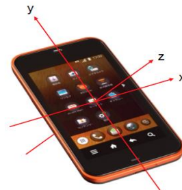
Figure 3. Axis of smartphone sensor
