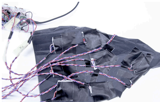
Figure 2: Pressure pads attached on the inner surface of the instrument
