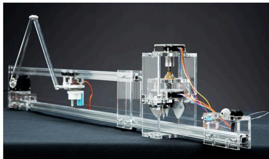
Figure 1: Protochord, a mechatronic monochord
