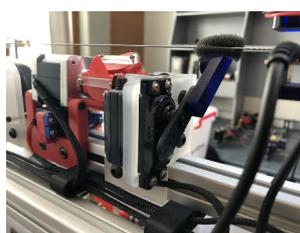
Figure 8: MechBass' servomotor-based damper
