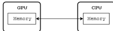
Figure 2: CPU to GPU memory accesses across system bus into respective device’s memory.
