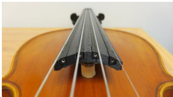
Figure 3. Front view of the end of the fingerboard without the Arduino and FSRs.
