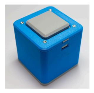
Figure 1: One of three one-button sound cubes.
