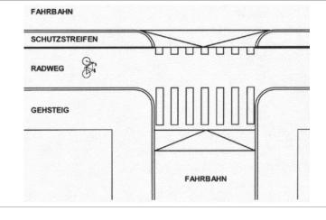
Figure 21: Example of an elevated road section at a Tjunction, which does not affect cyclists. (FSV 2014)
