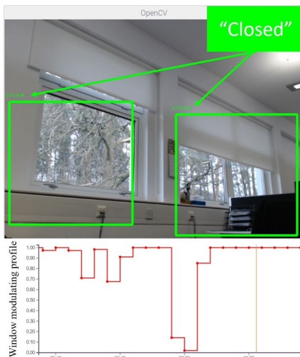
Fig. 1. Example of application of computer vision in the edge, using a script that is able to detect a window in the image and determine whether it is opened or closed (upper part), then the information is turned into time-series data (bottom part).
