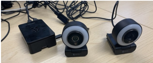
Fig. 4. Raspberry Pi 4 and standard webcams used for the experiment.
