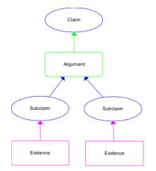
Figure 4: Example of CAE structure in an assurance case
