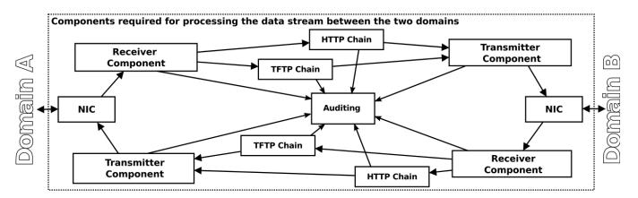
Figure 1: High-level View of Gateway Components
