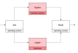
Figure 10. Software architecture of crypto controller system
